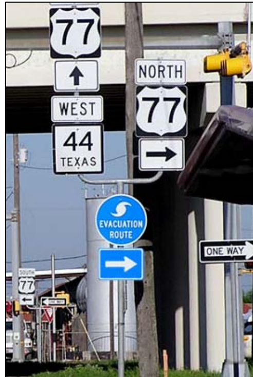
Figure 5. EM-1a Evacuation Route Sign with Supplemental Arrow
