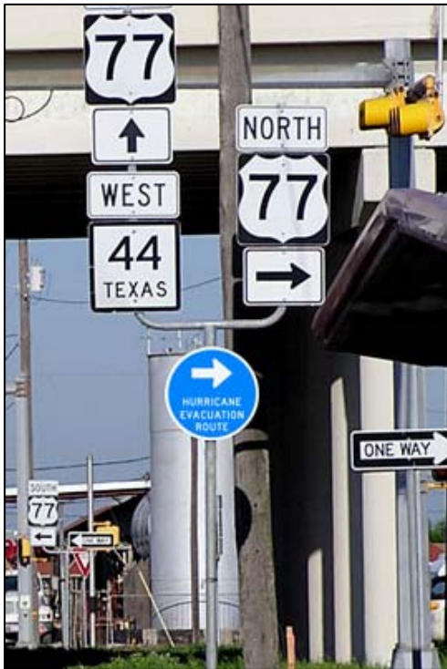
Figure 4. EM-1T Evacuation Route Sign
