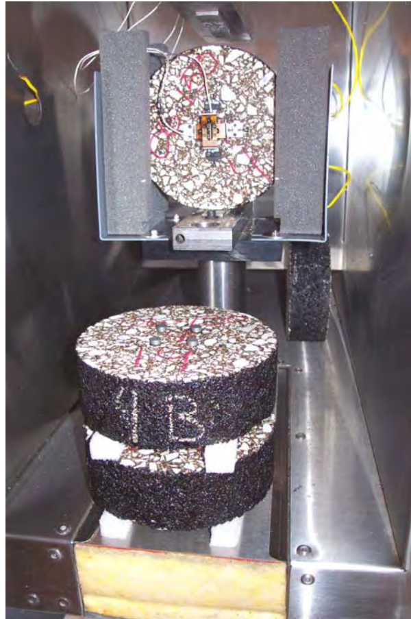
Figure 5: Low Temperature Tensile Strength Testing Configuration
