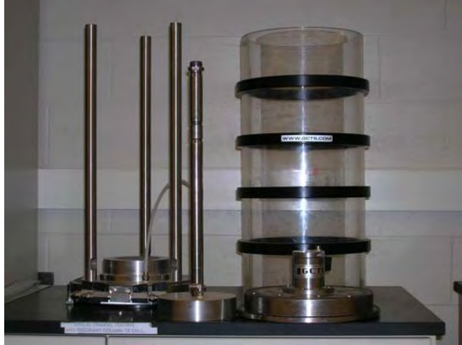
Figure 2.2 – GCTS 6-inch Diameter Triaxial Cell
