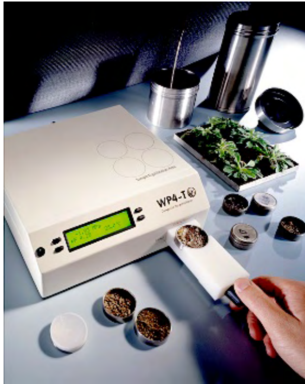
Figure 2.3 WP4 Potentiometer (Courtesy of Decagon Devices, Inc.)
