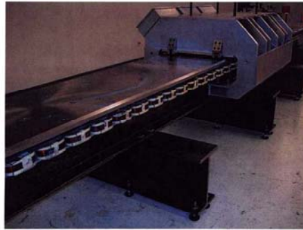
Figure 4. Photograph of the low speed prototype showing vehicle, guideway, and propulsion coils (laboratory demonstration)
