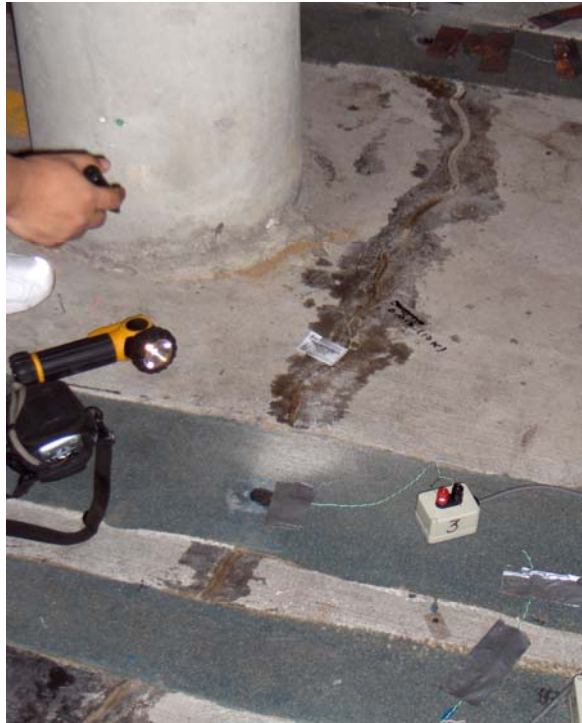
Figure 5.8: CFRP Strengthening Subjected to the Design Load
