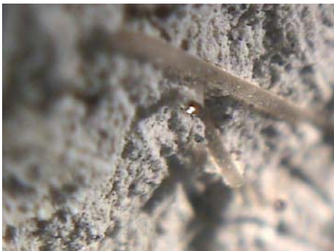
Figure 7: SIP-120 in cement after 2 days (left) and after 28 days (right)
