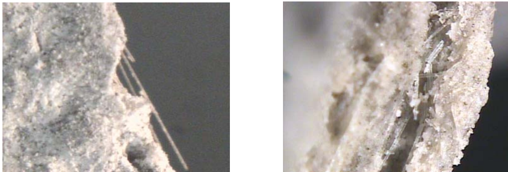
Figure 19: Optical micrographs of the fracture surfaces of GFRC coupons made with uncoated SIP-91 glass fibers after curing for 7 days (left) and 28 days (right).
