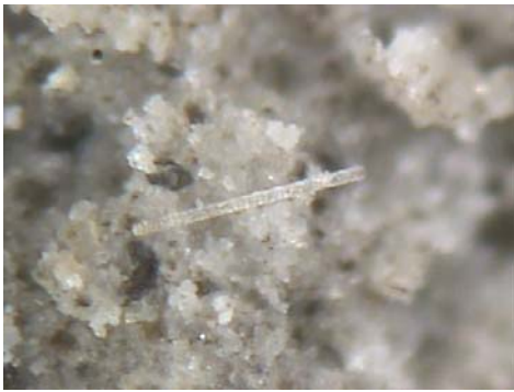
Figure 6: SIP-91 in cement after 2 days (left) and after 28 days (right)
