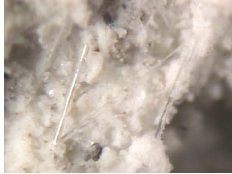
Figure 5: Uncoated Cem-FIL fibers in cement after 2 days (left) and after 28 days (right).
