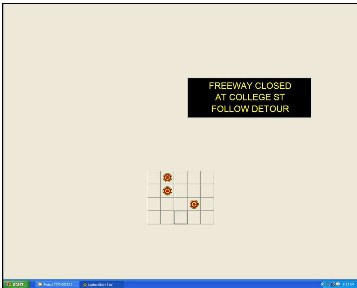
Figure 8. Screen Capture of the Personal Computer Study Procedure Showing On-Screen Changeable Message Sign and Control Panel Monitoring Secondary Task
