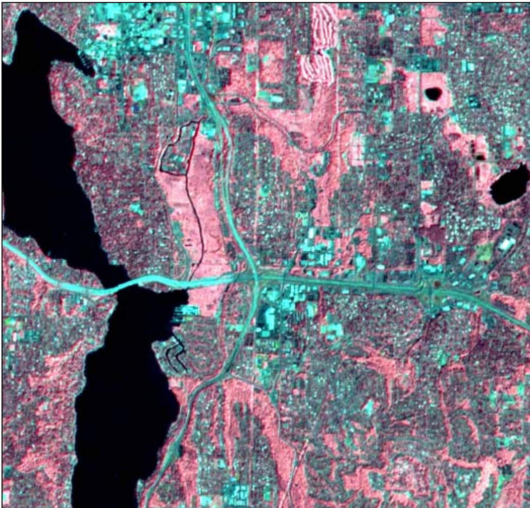
Figure 3.1. Landsat ETM+ Multispectral Imagery Shows the Intersection of I-405 and I-90. Graphical Display Generated with Landsat ETM+ Band 4 (Red), Band 3 (Green) and Band 2 (Blue) Sharpened to 15 Meter Resolution Using the ETM+ Panchromatic Band.
