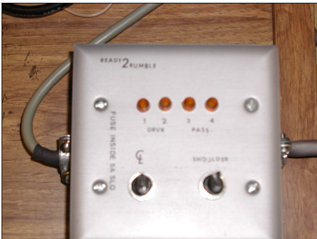
FIGURE 17. Ready2Rumble Control Box to Activate the Vibratory Motors.
