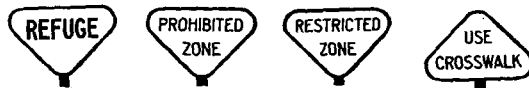
FIGURE 7. Security Signs, primarily for pedestrians. Blue letters and borders on white ground.
