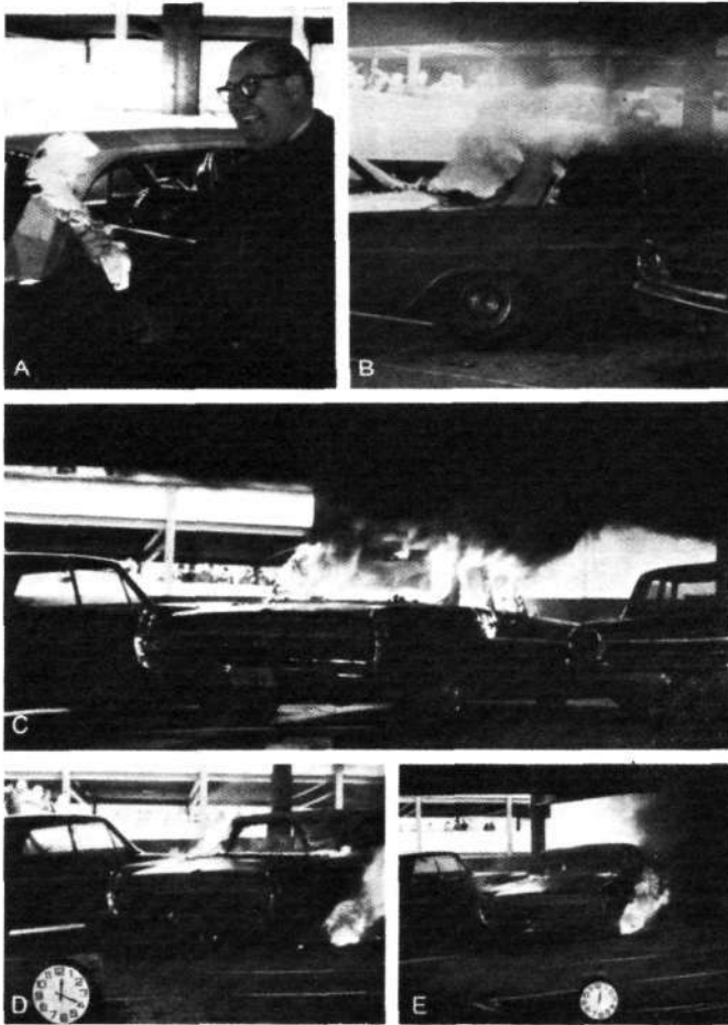
FIGURE 33. The Scranton Fire Test, Municipal Parking Structure, Scranton, Pennsylvania, October 15, 1972.
