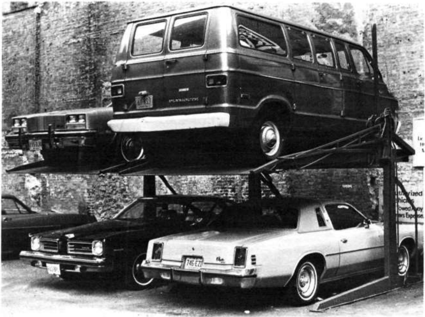
FIGURE 13. Parking devices such as this can increase parking for very limited land areas.
