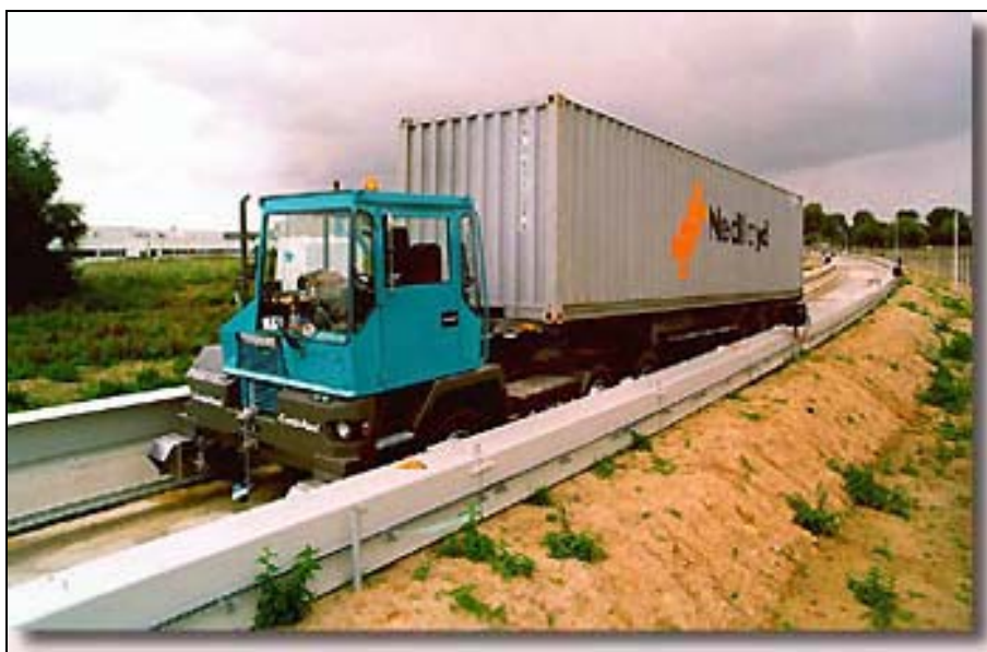
Figure 8-17: Combi-Road Driverless Truck Guideway
