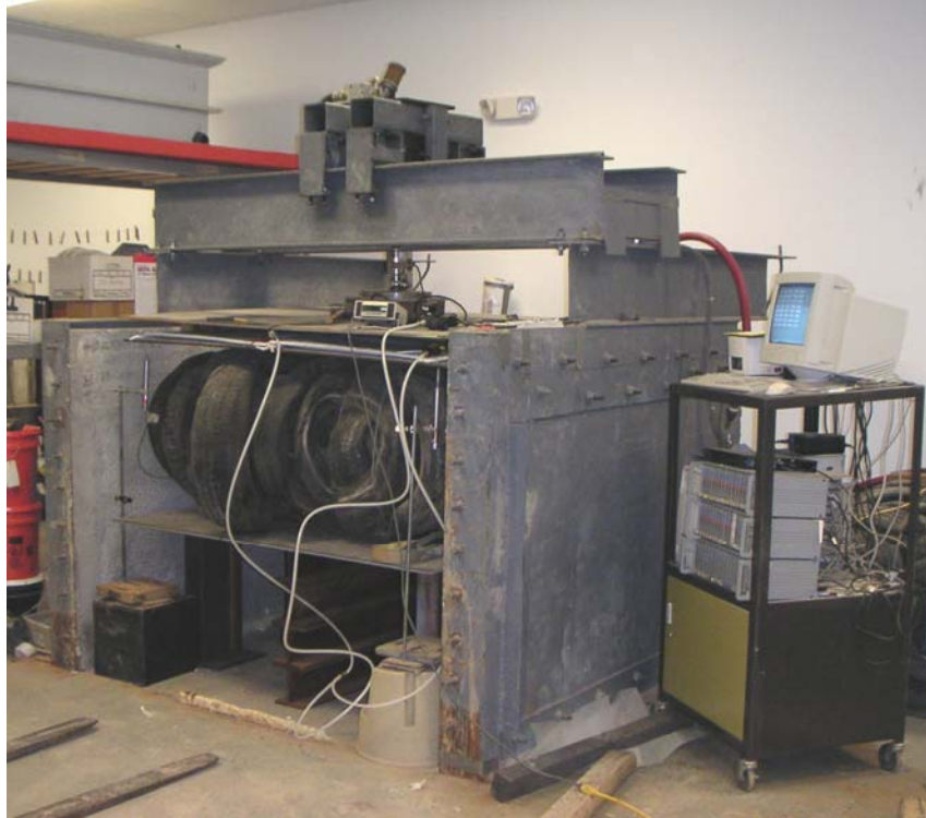
Figure 4.5. Creep test setup.
