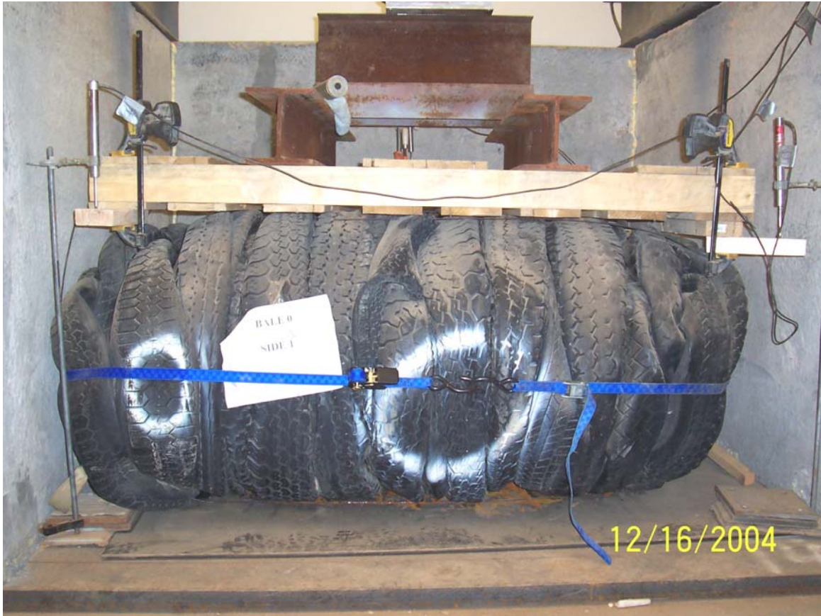
Figure 4.8. Rebound test on tire bales showing lateral expansion in the first test
