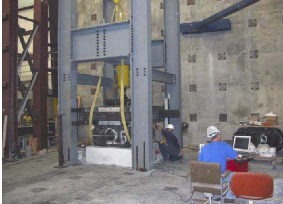
Figure 4.1 Typical tire bale compression test setup
