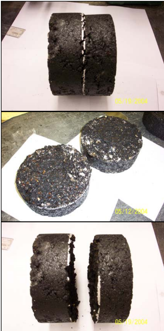
Figure 3.8 Fully Sheared Interface Specimen.
