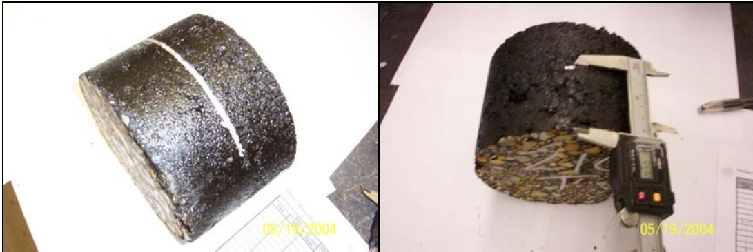
Figure 3.6 Locating the Interface of Shear Specimens
