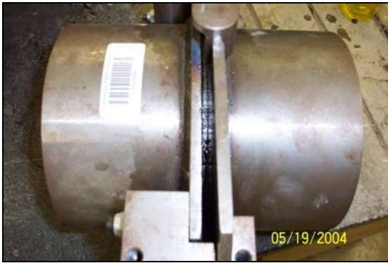
Figure 3.7 Correct Alignment of Specimens.
