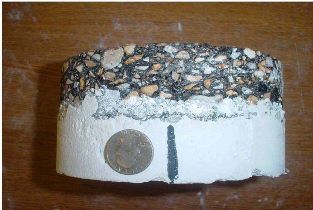
Figure 3.6 Core After Plastering.
