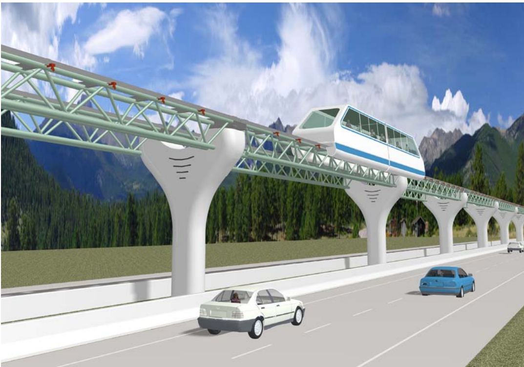
Figure A-11: Concept C: Rendering of Steel Truss Guideway
