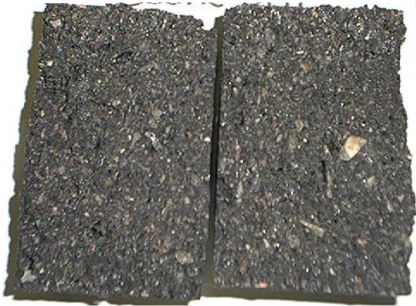
Figure 5.2 – TSR Specimen Failure: 5% Boone BHF, 0% LOF
