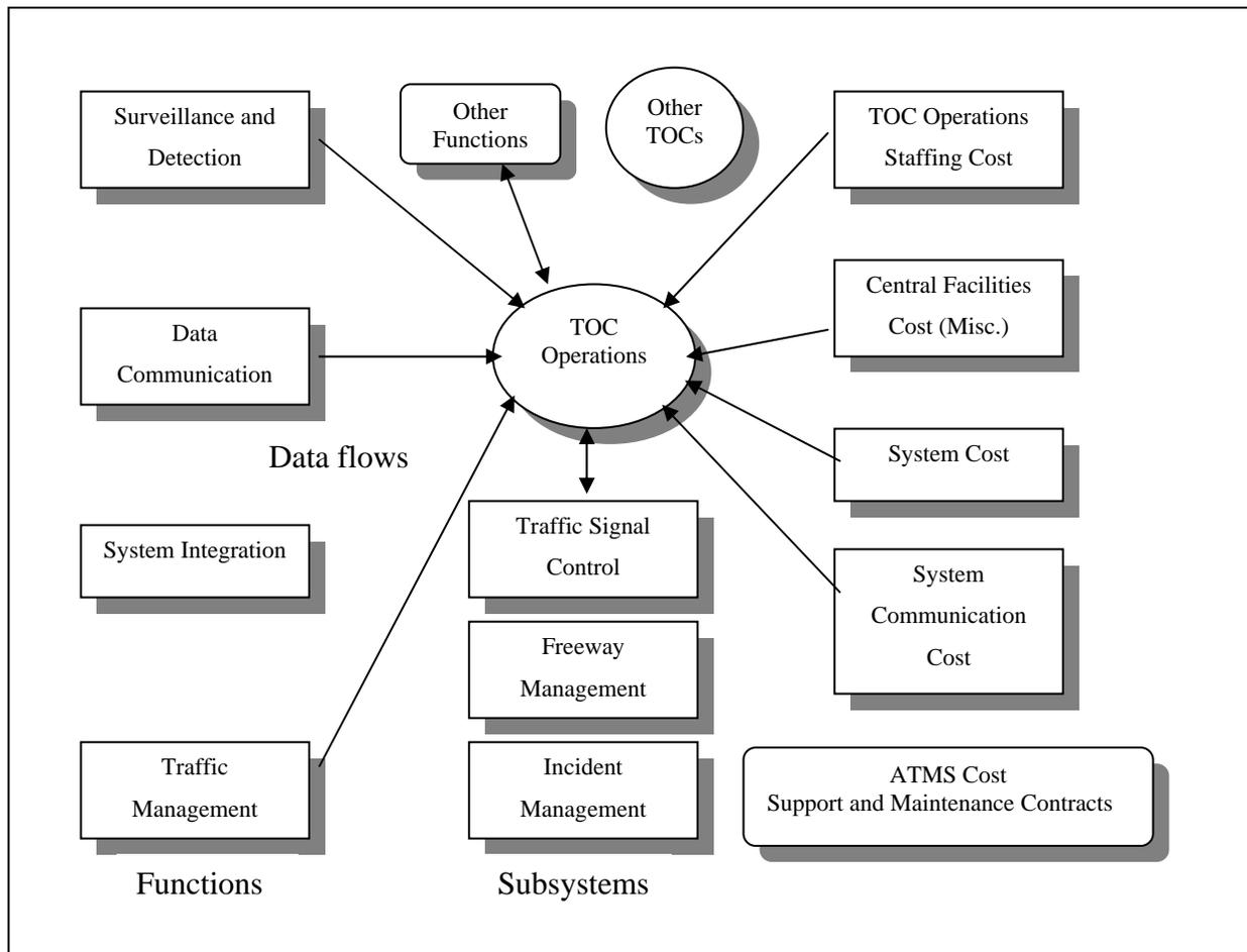
**Figure 3. Typical Functions Performed by Other States' TOCs.**
