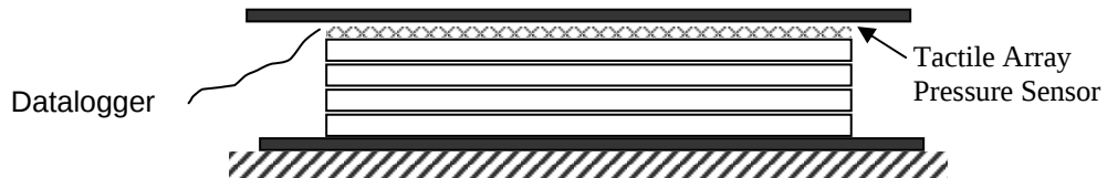
Figure 2.8. Bearing Instrumentation using Tactile Pressure Sensor
