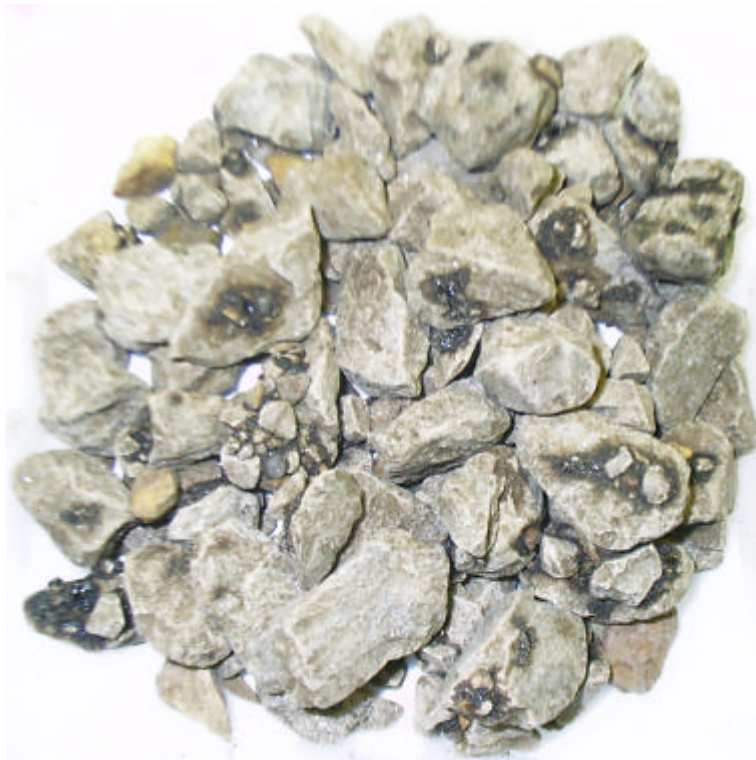
Figure 5.12 Partial Extraction Residue of Mix-E
