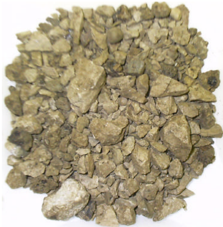
Figure 6.14 Partial Extraction Residue of Mix-LB (15% RAP) Comparison Sample
