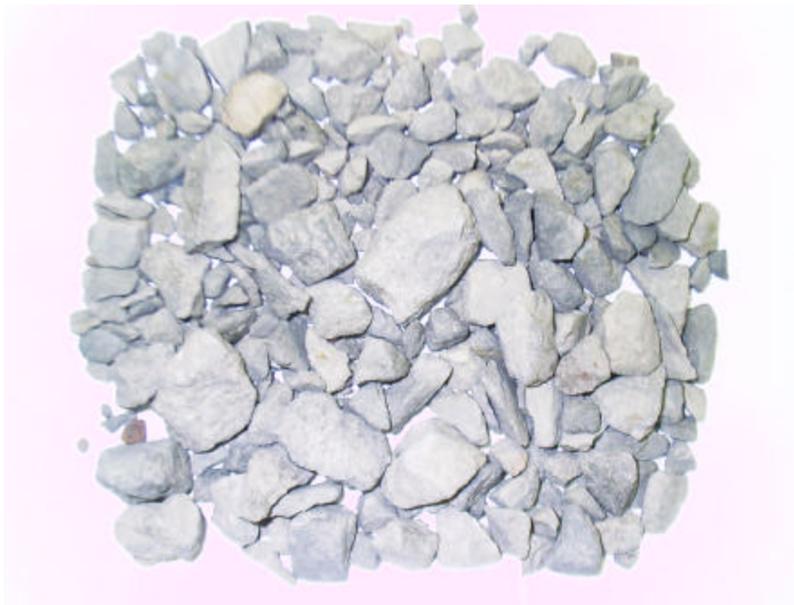
Figure 5.14 Portion of Mix-C Partial Ignition Residue without Binder Traces
