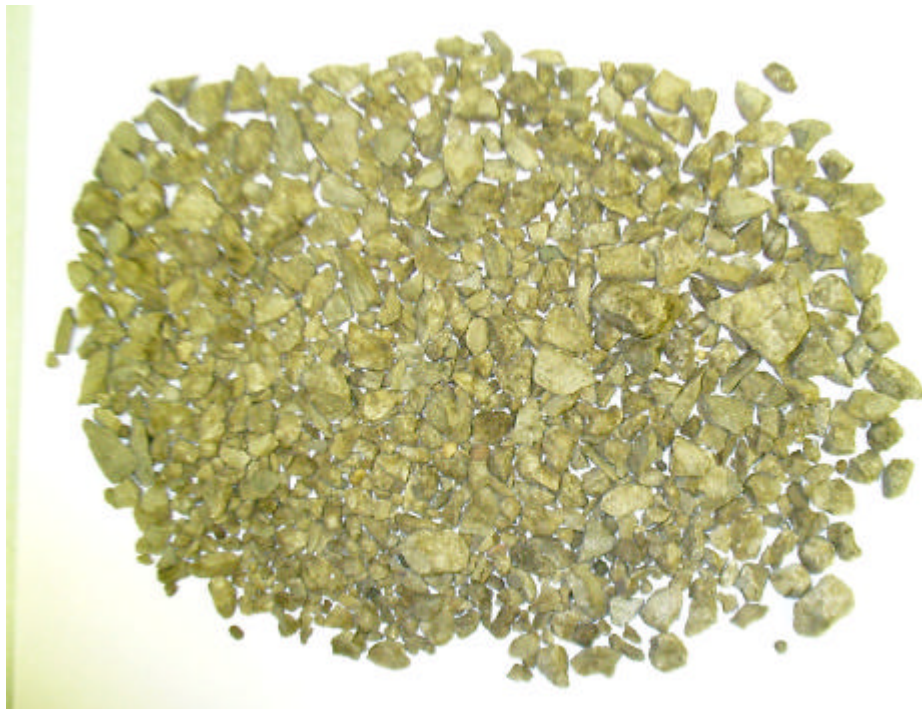
Figure 8.3 Partial Extraction Residue for Virgin Mix-2 Indicating the Absence of RAP
