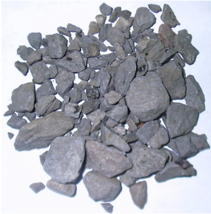
Figure 5.2 Partial Extraction Residue for Mix-C (Initial Soaking Time = 90-min, Initial Solvent = 50% Toluene, Final Soaking Time = 30-sec, Final Solvent = 85% Toluene)
