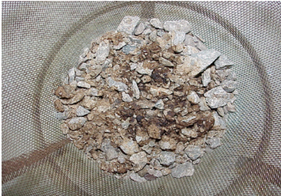
Figure 4.6 Partially Extracted Sample of Bituminous Mixture with 30% RAP
