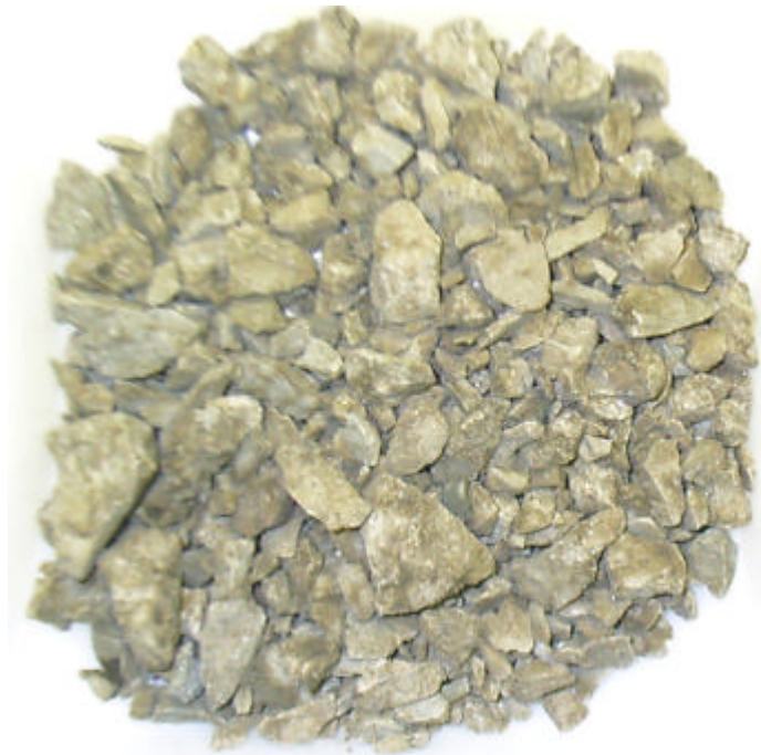
Figure 6.8 Partial Extraction Residue of Mix-LA (0% RAP) Comparison Sample
