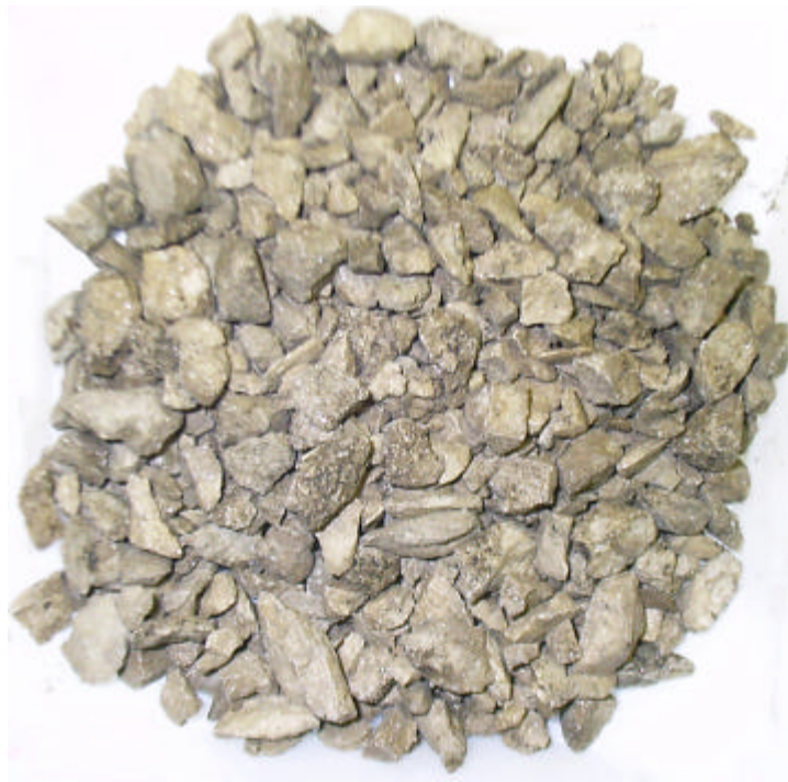
Figure 6.22 Partial Extraction Residue of Mix-F (0% RAP) Comparison Sample
