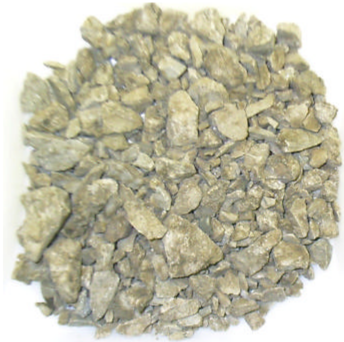
Figure 8.6 Partial Extraction Residue of Mix-LA (0% RAP) Comparison Sample
