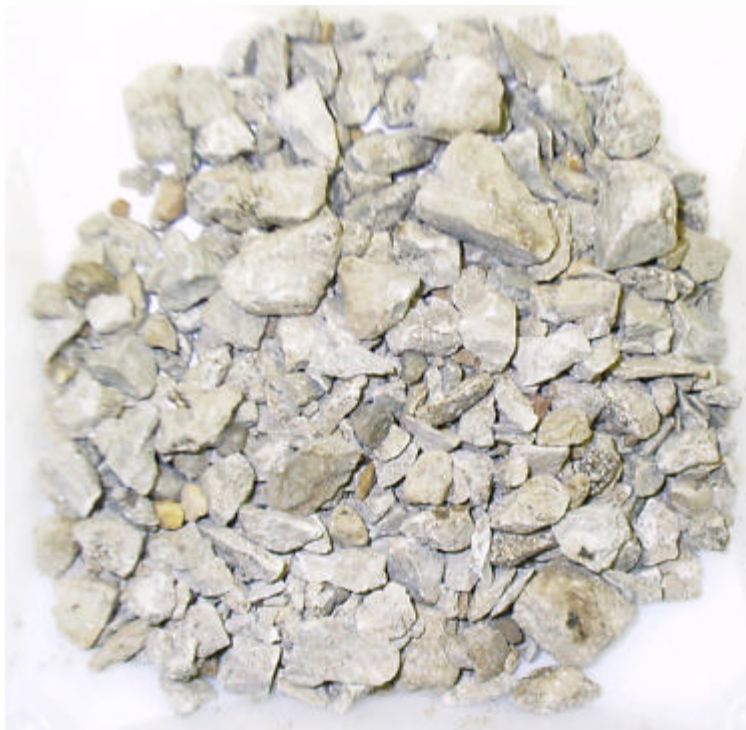
Figure 6.13 Partial Extraction Residue of Mix-LB (0% RAP) Comparison Sample
