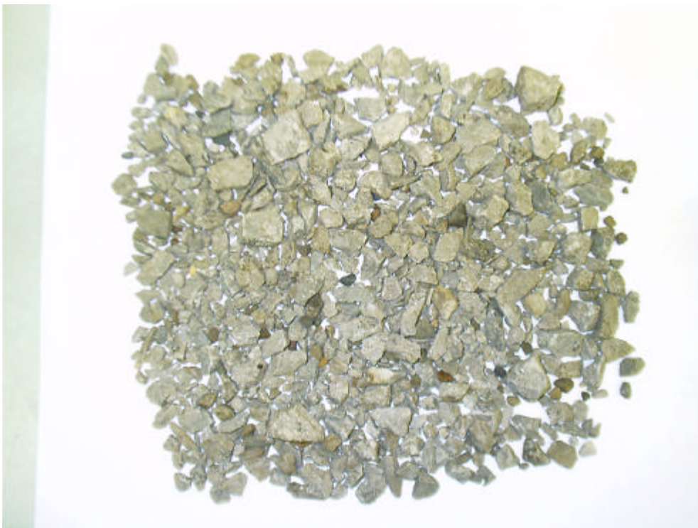
Figure 5.8 Partial Extraction Residue of Virgin Mix-3 (No RAP)
