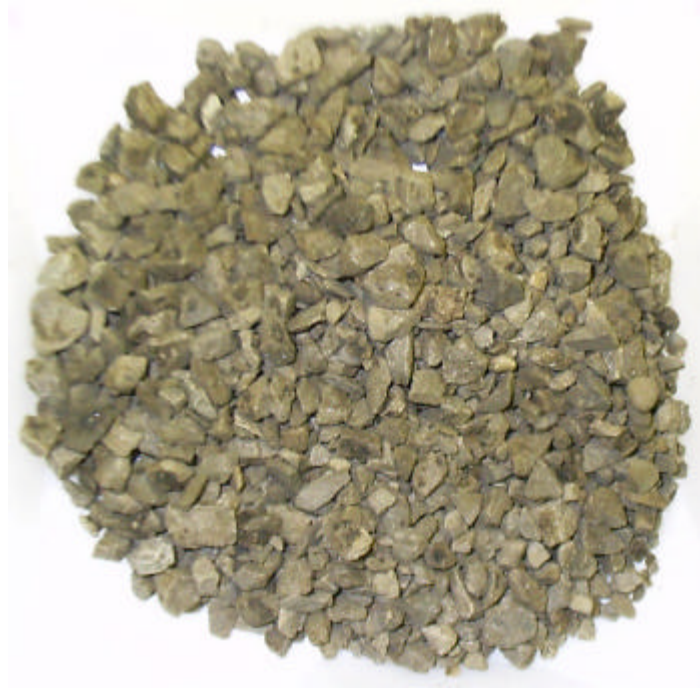
Figure 6.11 Partial Extraction Residue of Mix-LA (100% RAP) Comparison Sample
