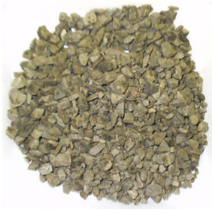
Figure 8.9 Partial Extraction Residue of Mix-LA (100% RAP) Comparison Sample
