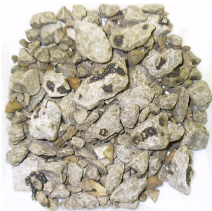
Figure 6.21 Partial Extraction Residue of Mix-E (Field Core) Sample (20% RAP)
