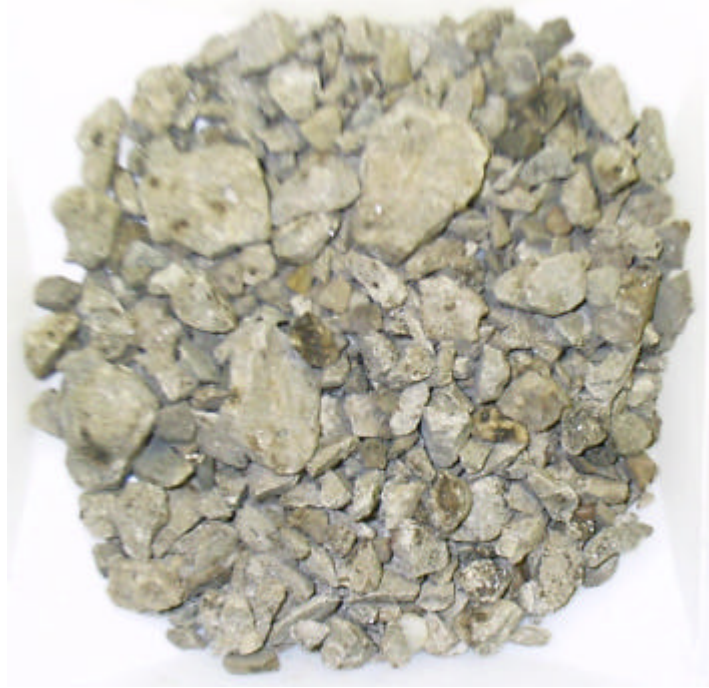
Figure 8.7 Partial Extraction Residue of Mix-LA (15% RAP) Comparison Sample
