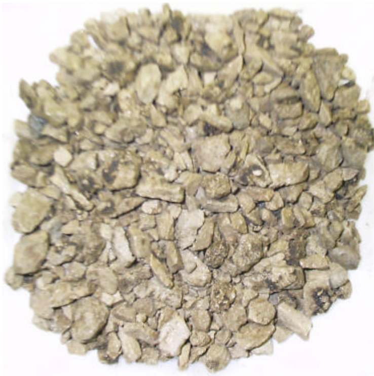
Figure 6.24 Partial Extraction Residue of Mix-F (Plant Mix) Sample (10% RAP)
