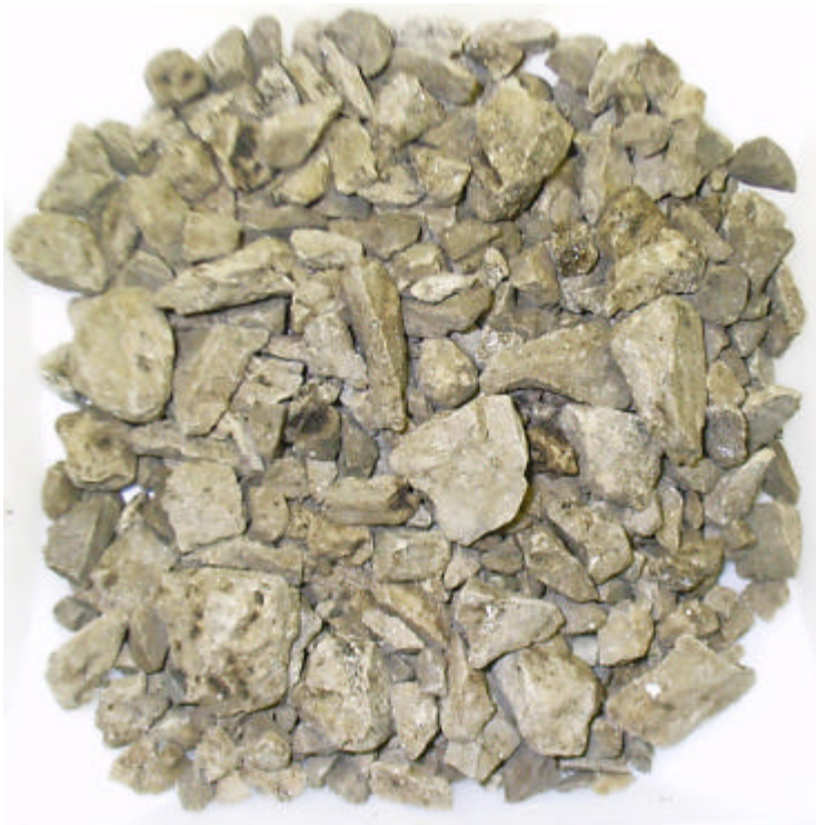
Figure 6.9 Partial Extraction Residue of Mix-LA (15% RAP) Comparison Sample
