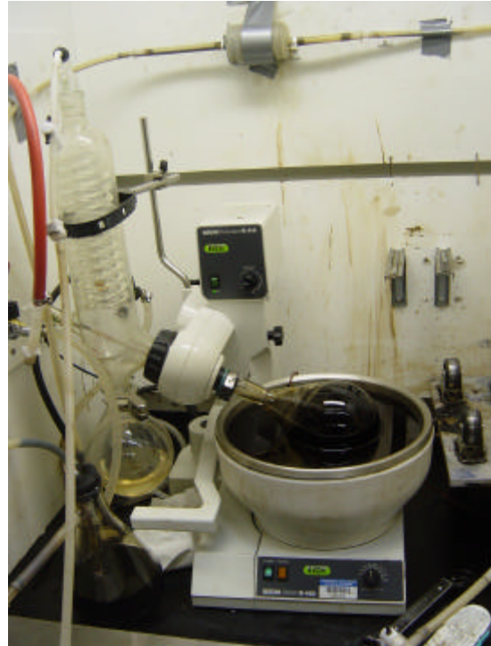
Figure 4.8 Recovery Equipment ( Roto-Vap Unit )
