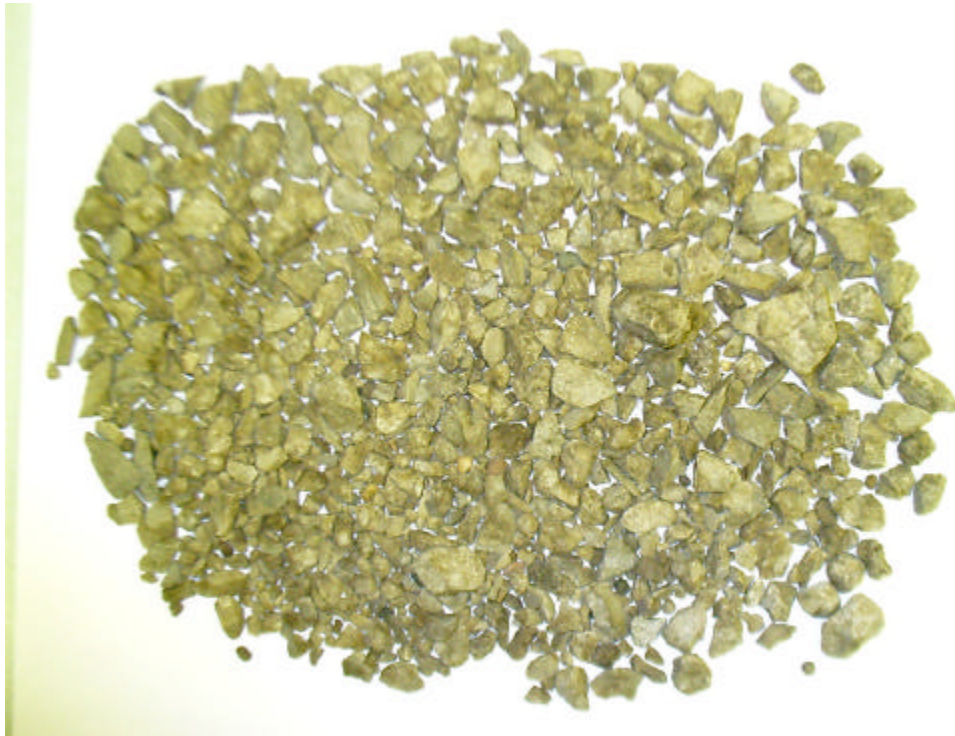
Figure 5.7 Partial Extraction Residue of Virgin Mix-2 (No RAP)
