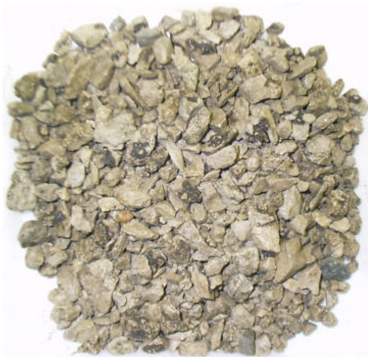
Figure 6.25 Partial Extraction Residue of Mix-F (Field Core) Sample (10% RAP)
