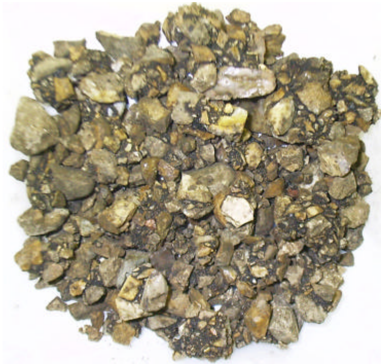
Figure 6.19 Partial Extraction Residue of Mix-E (100% RAP) Comparison Sample
