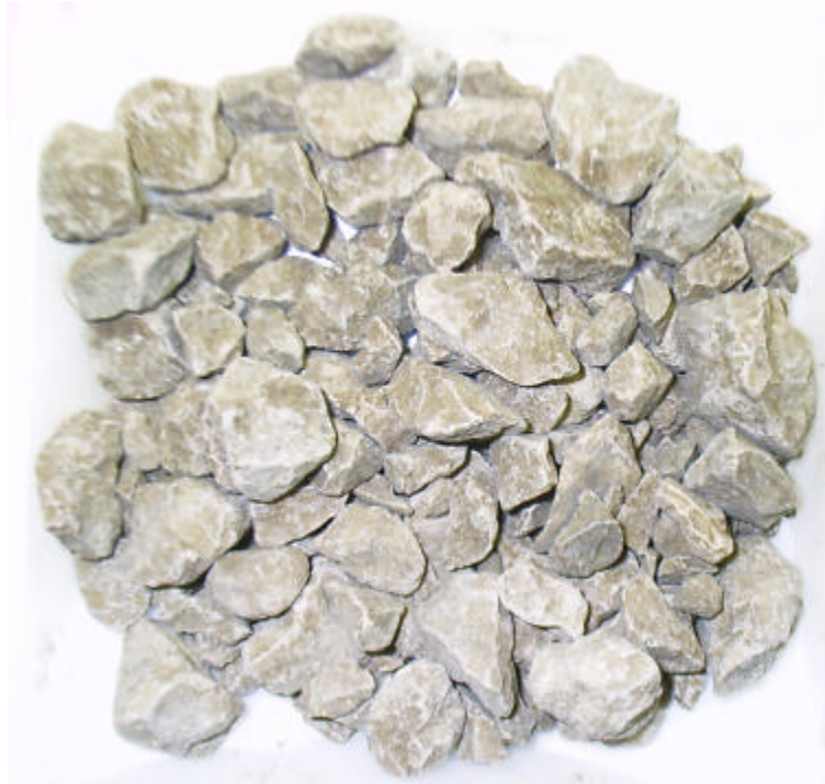
Figure 6.18 Partial Extraction Residue of Mix-E (0% RAP) Comparison Sample
