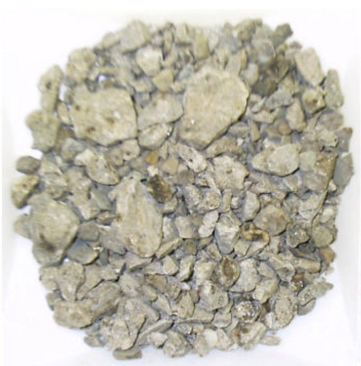
Figure 6.9 Partial Extraction Residue of Mix-LA (15% RAP) Comparison Sample
