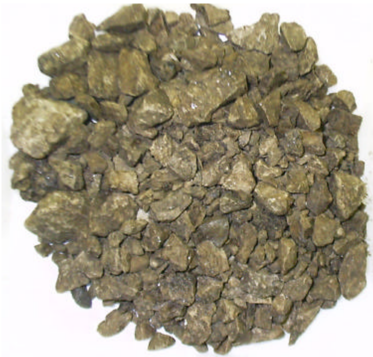
Figure 6.15 Partial Extraction Residue of Mix-LB (30% RAP) Comparison Sample
