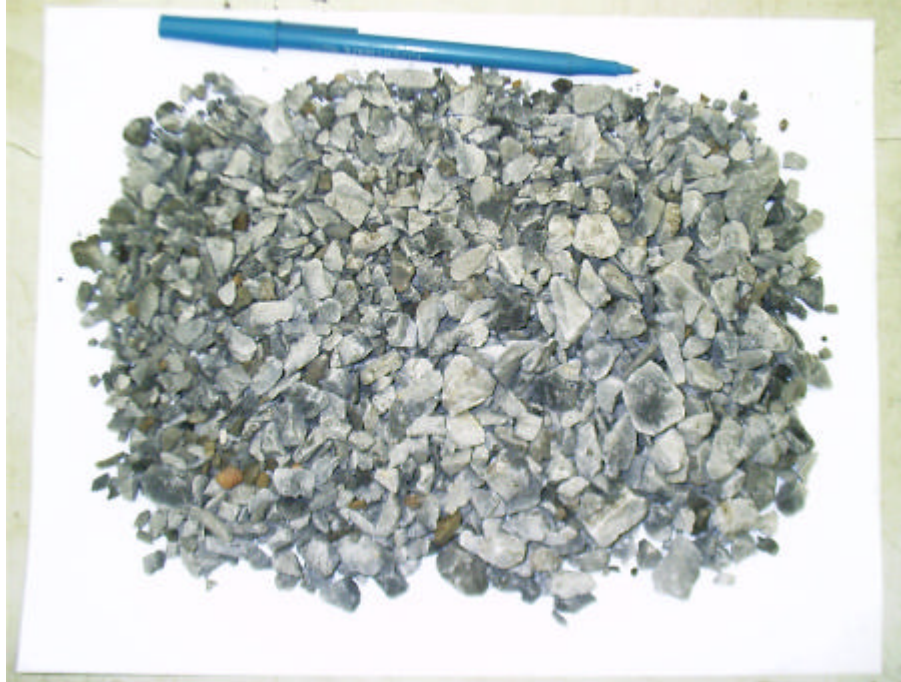
Figure 5.17 Low Temperature Partial Ignition of Virgin Mix-2 (400°C)
