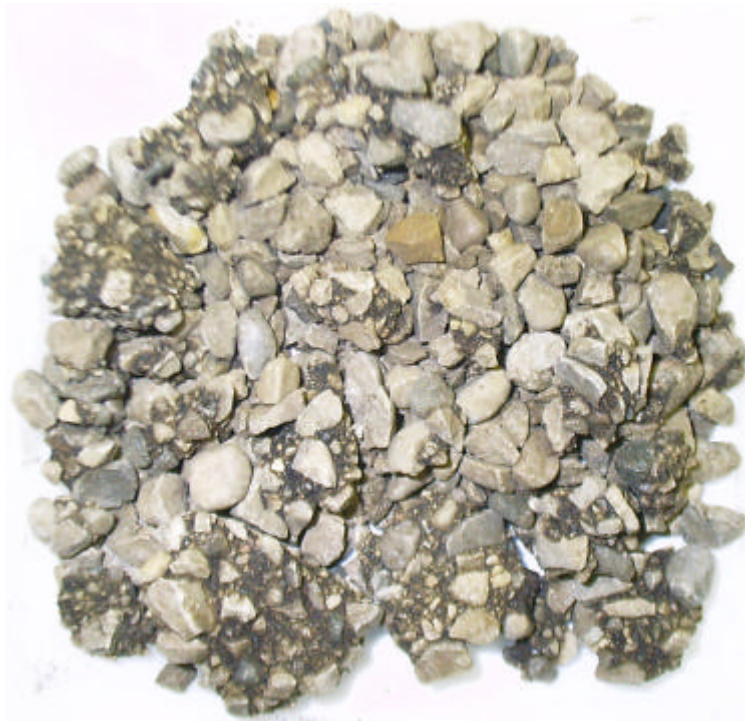
Figure 6.23 Partial Extraction Residue of Mix-F (100% RAP) Comparison Sample
