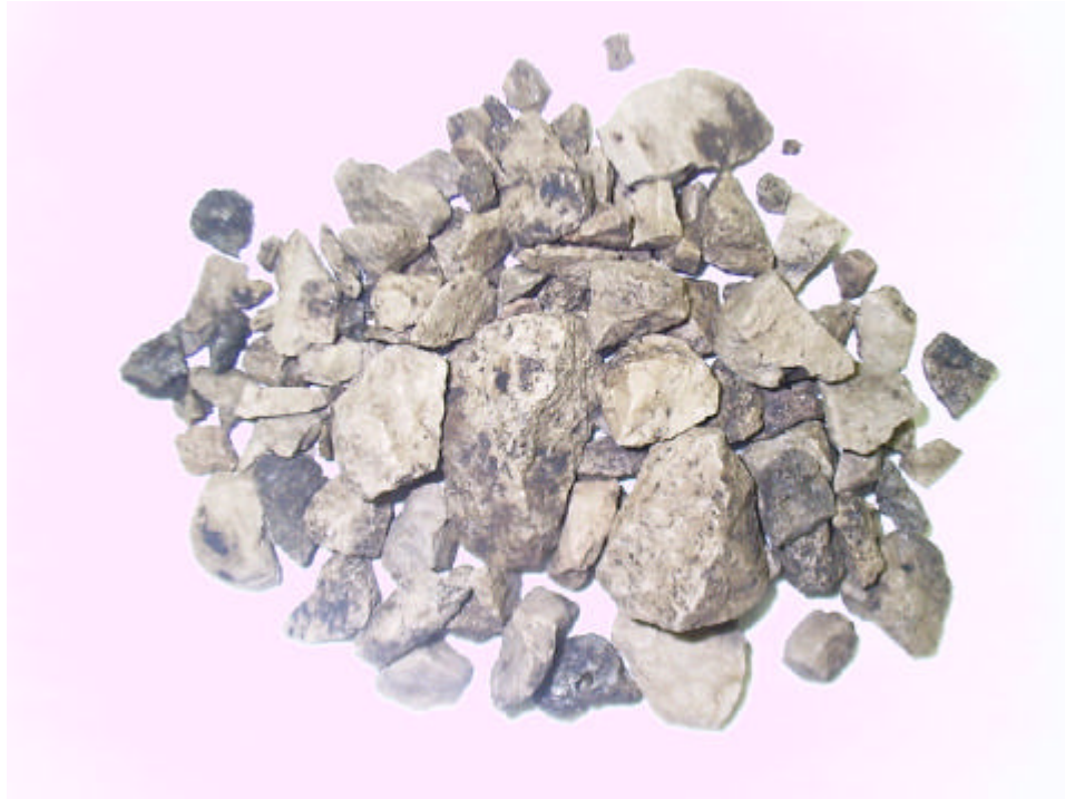
Figure 5.1 Partial Extraction Residue for Mix-C (2-hour soaking with 70% Toluene)
