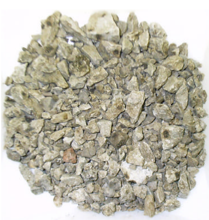
Figure 8.10 Partial Extraction Residue of Mix-LA Unknown RAP Sample (22.5% RAP)
