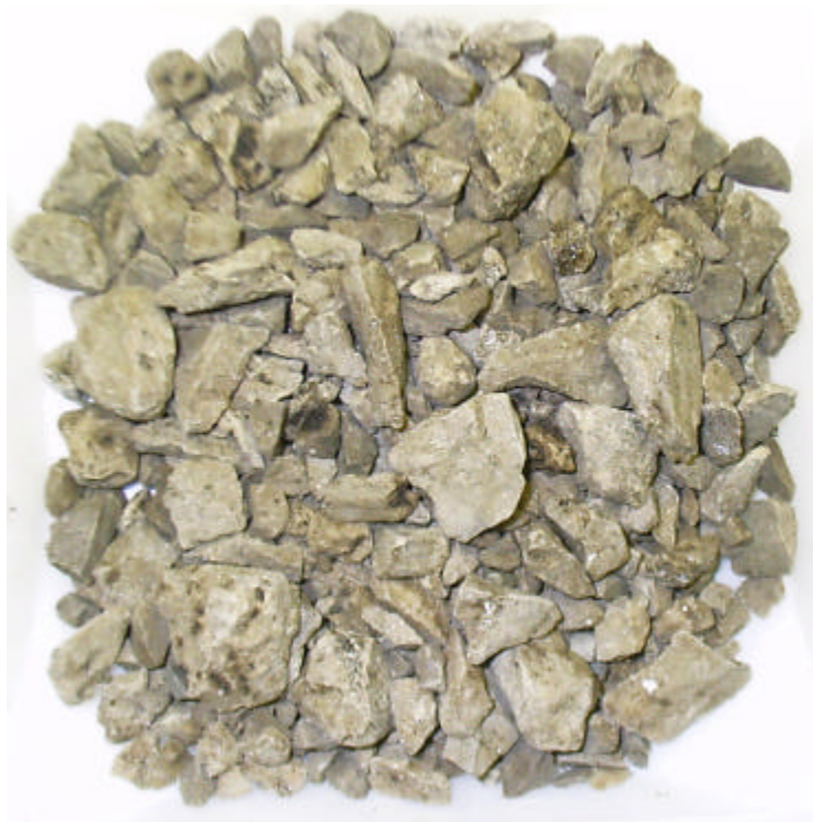
Figure 8.8 Partial Extraction Residue of Mix-LA (30% RAP) Comparison Sample
