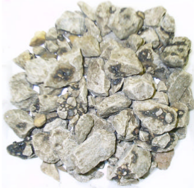
Figure 8.4 Partial Extraction Residue of Mix-E Indicating the Presence of RAP (10% RAP was Present in the Actual Mix)
