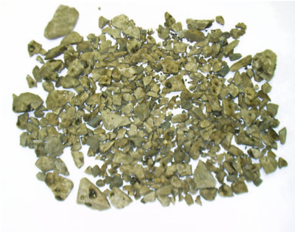
Figure 7.6 Partially Extracted Mix with 20% RAP-3 (Softest)
