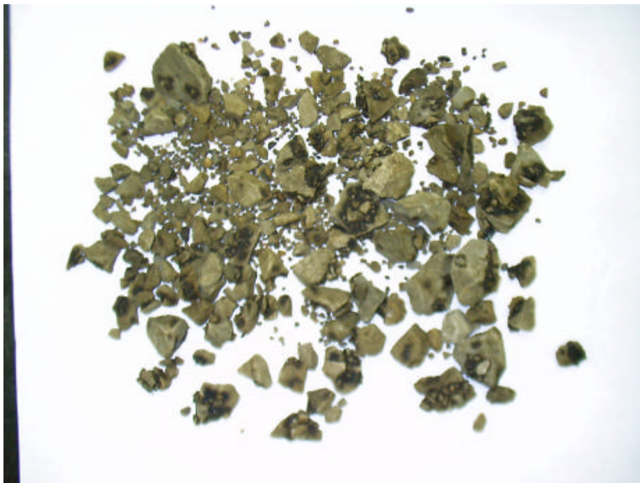
Figure 5.10 Partial Extraction Residue of Mix-B (29.5% RAP)
