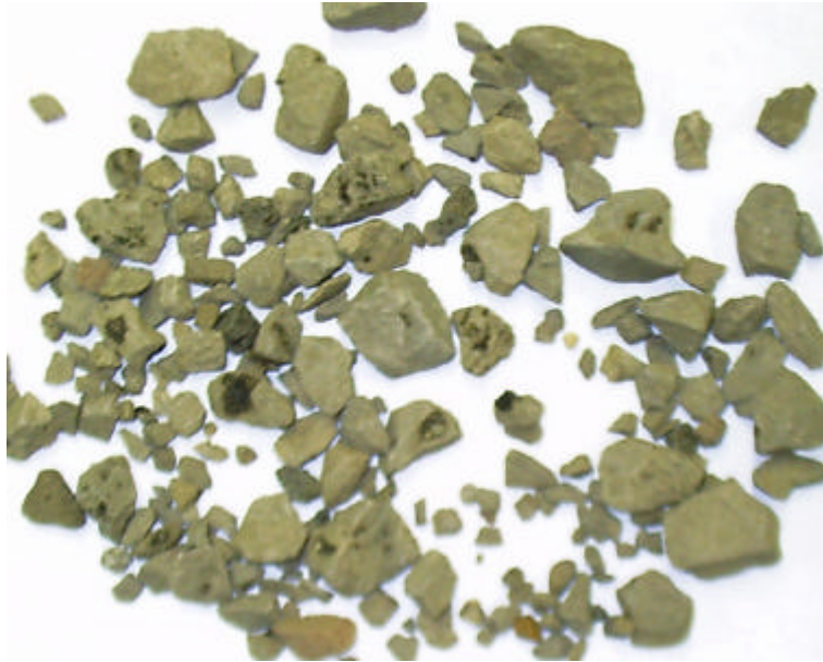
Figure 5.3 Partial Extraction Residue for Mix-C (Initial Soaking Time = 120-min, Initial Solvent = 50% Methylene Chloride, Final Soaking Time = 1-min, Final Solvent = 85% Methylene Chloride)
