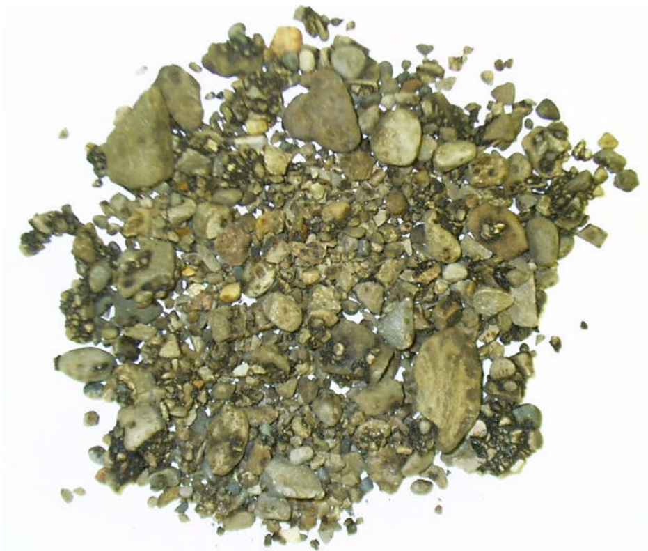
Figure 5.11 Partial Extraction Residue of Mix-D (29.3% RAP)
