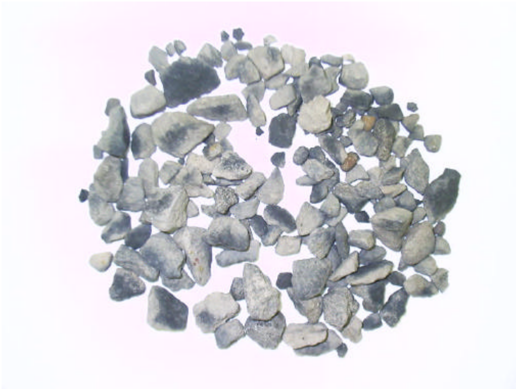
Figure 5.15 Portion of Mix-C Partial Ignition Residue with Binder Traces
