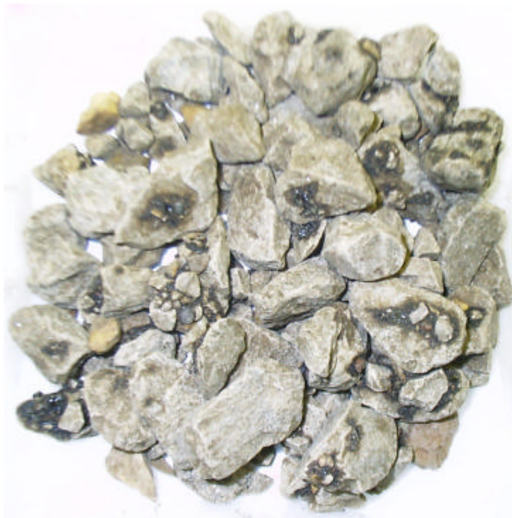
Figure 6.20 Partial Extraction Residue of Mix-E (Plant Mix) Sample (20% RAP)
