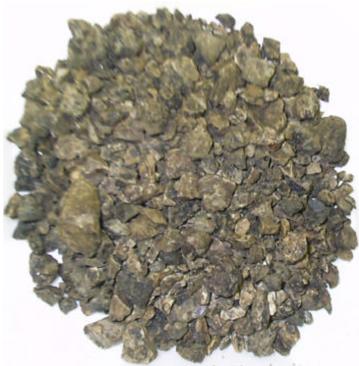
Figure 6.16 Partial Extraction Residue of Mix-LB (100% RAP) Comparison Sample
