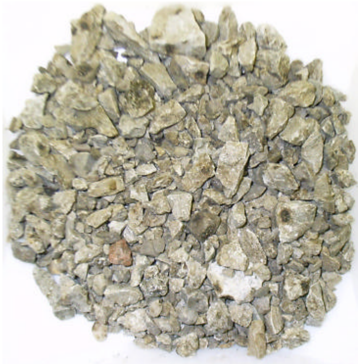
Figure 6.12 Partial Extraction Residue of Mix-LA Candidate RAP Sample (22.5% RAP)
