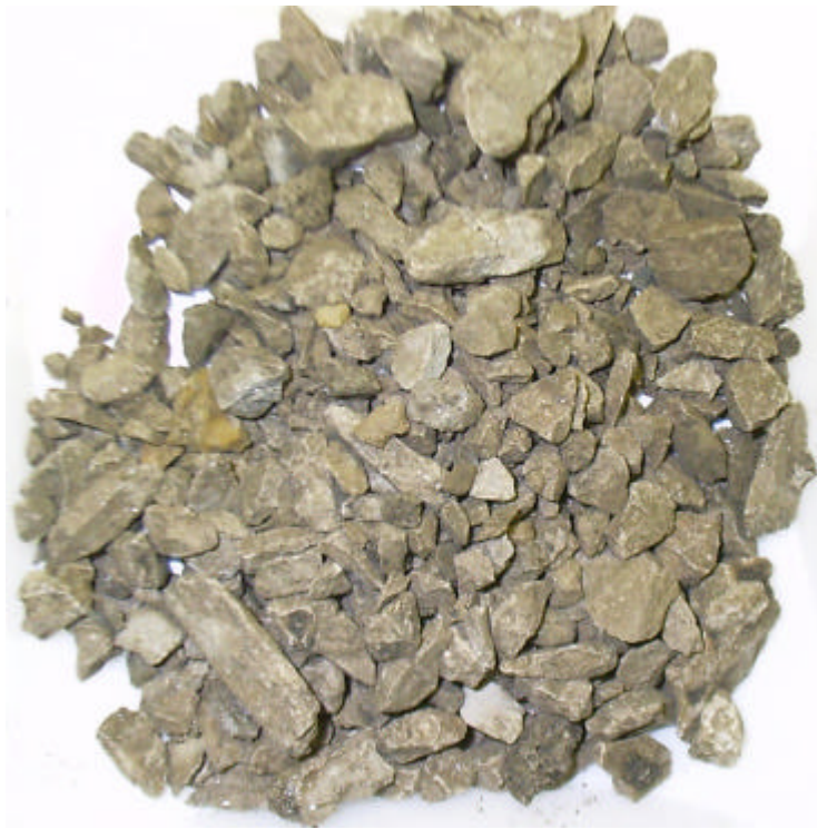
Figure 6.17 Partial Extraction Residue of Mix-LB Candidate RAP Sample (12.5% RAP)
