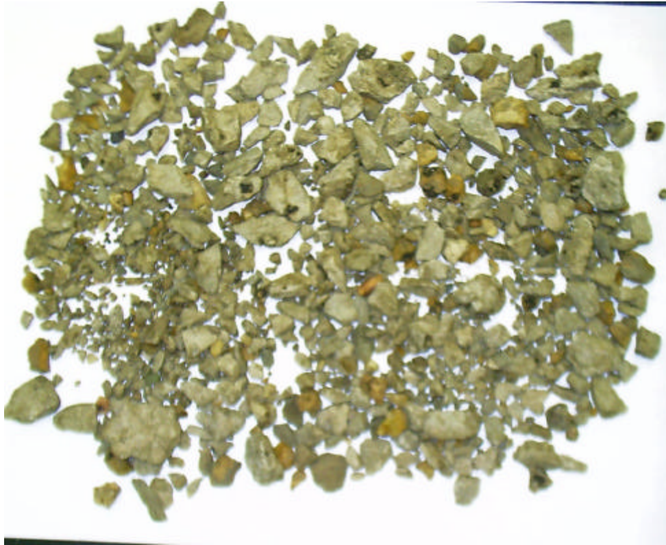
Figure 7.7 Partially Extracted Mix with 20% RAP-8 (Stiffest)
