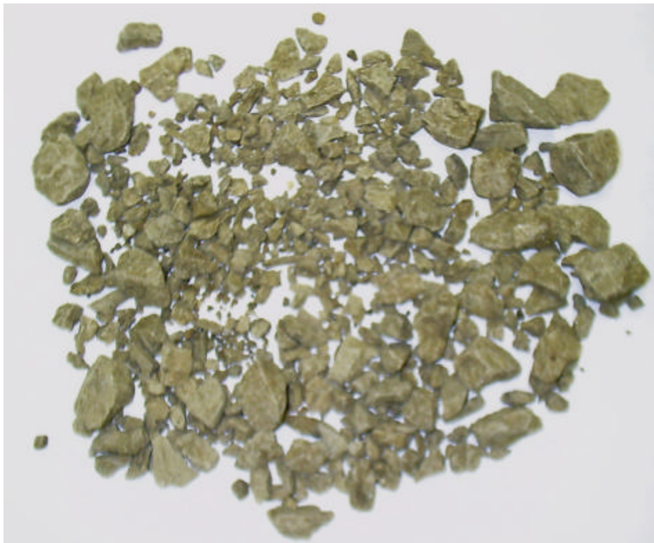
Figure 5.6 Partial Extraction Residue of Virgin Mix-1 (No RAP)
