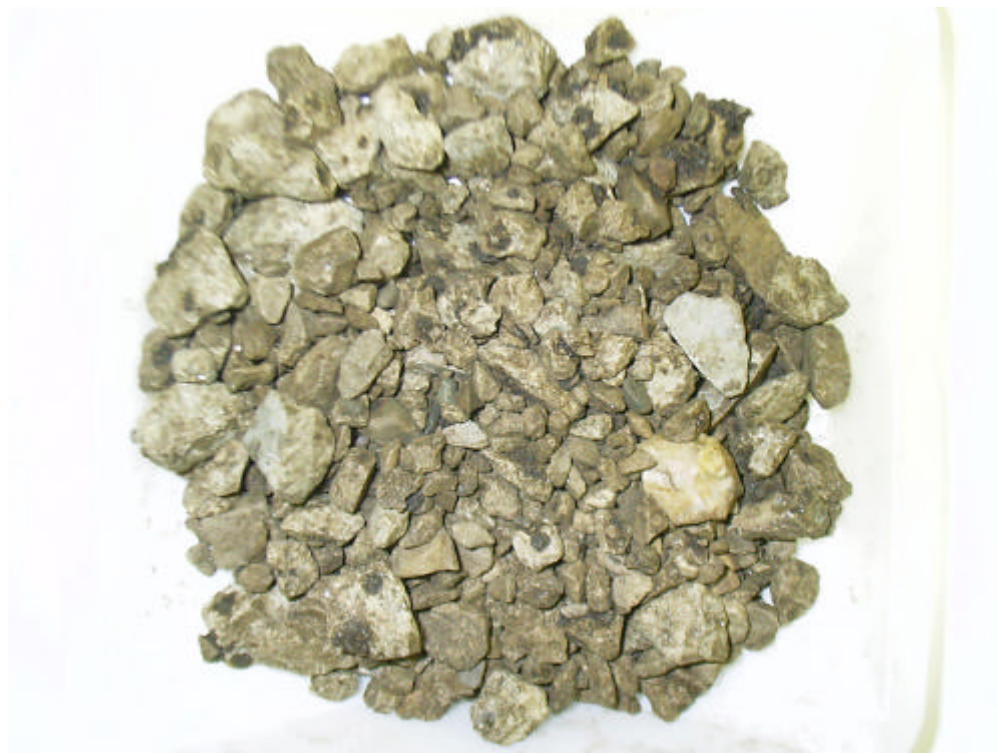
Figure 8.14 Partial Extraction Residue for Mix-BS2
