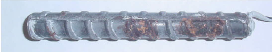
FIGURE 3.14: MMFX anode bar after removal of mortar, at 15 weeks
