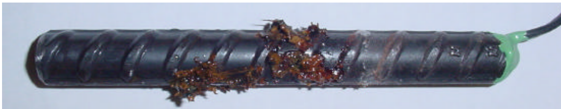
FIGURE 3.12: Bare MMFX anode bar from group MMFX (2), at 15 weeks, showing corrosion products that formed below the surface of the solution
