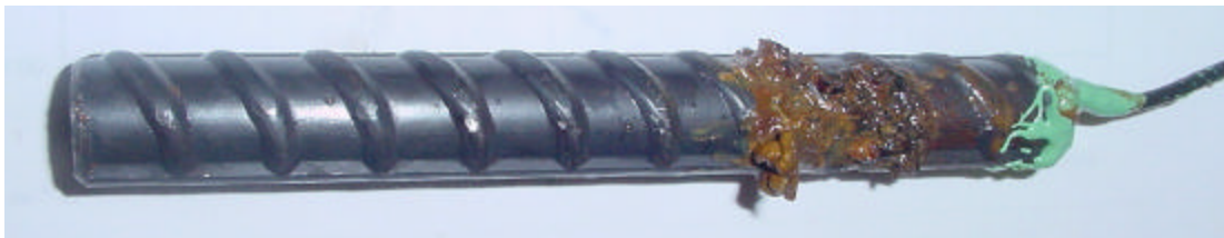
FIGURE 3.11: Bare MMFX anode bar from group MMFX (1), at 15 weeks, showing corrosion products that formed above the surface of the solution
