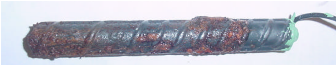
FIGURE 3.10: Bare conventional N3 anode bar, at 15 weeks
