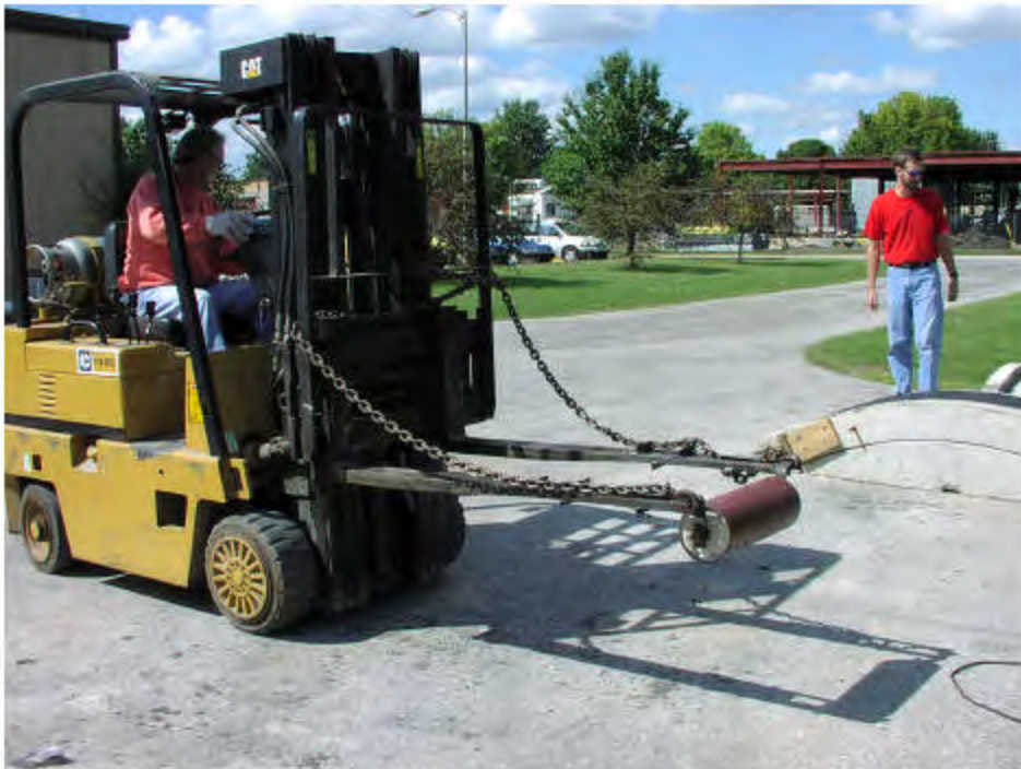
Figure B5 Forklift mounted rolling pin for greater force
