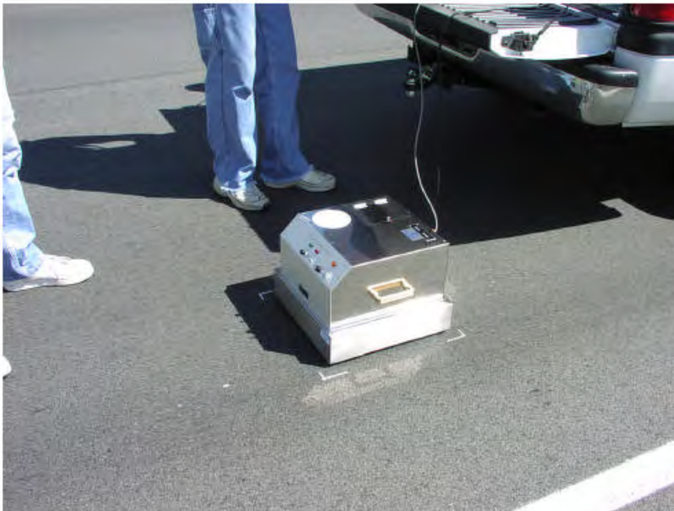
Figure B3 Measuring texture with Circular Track Meter
