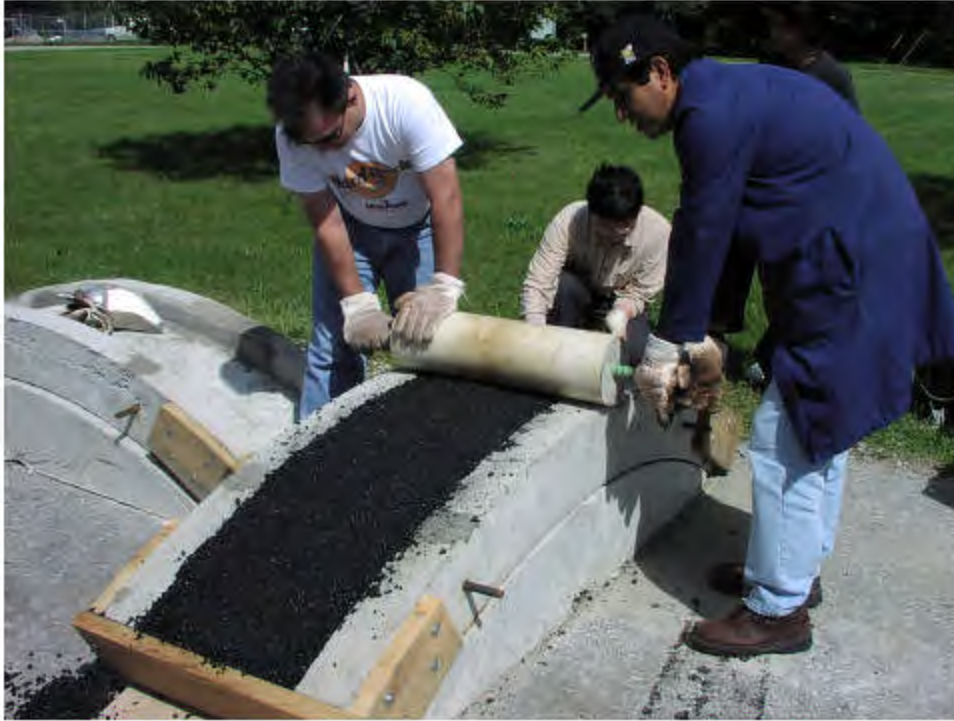
Figure B4 Compacting noise testing slabs with manual rolling pin
