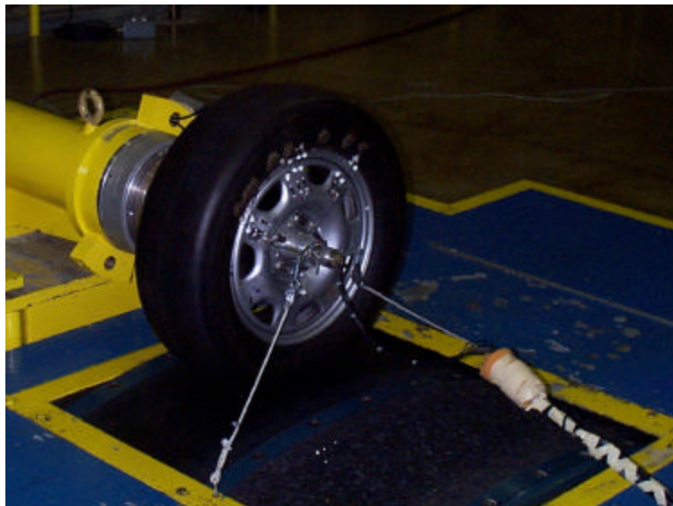
Figure 2-11: Goodyear test setup with tire on road wheel.
