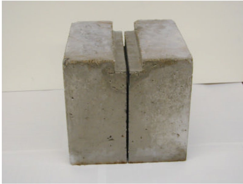
Figure 2.1 Picture of a wedge splitting test specimen
