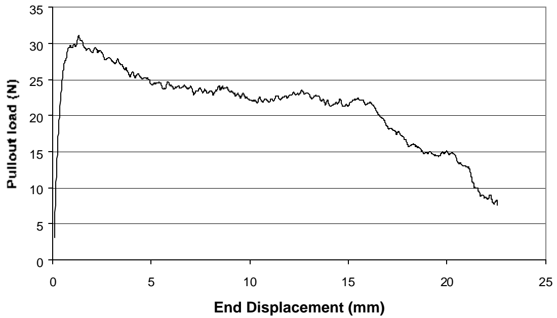
Figure 1.6. A typical Pullout of curve of Strux 85/80 fiber
