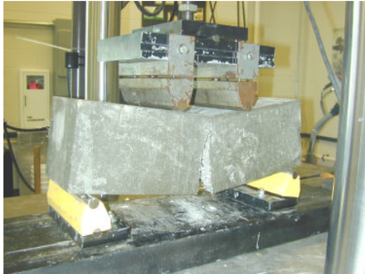
Figure 3. Failure of a beam in flexure
