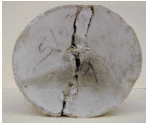
Figure 2. Failure mode under tensile splitting load
