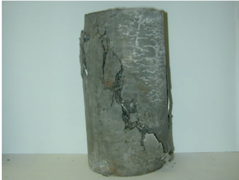
Figure 1. Failure mode in compression
