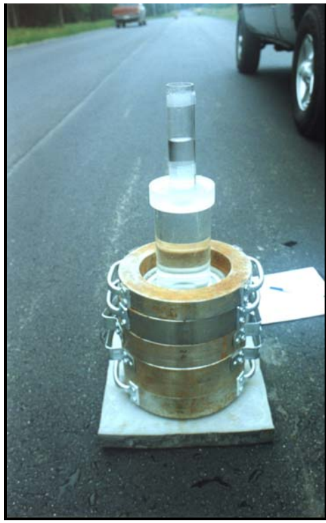
Figure 2. Sketch and Photo of Permeameter
