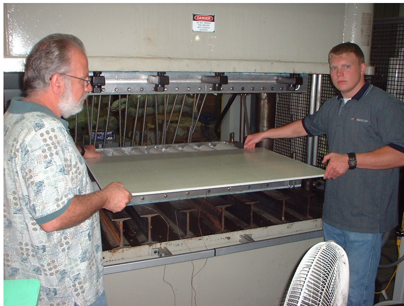
Figure 4.3.2-4 Placement of Secondary Part to be Adhesively Bonded
