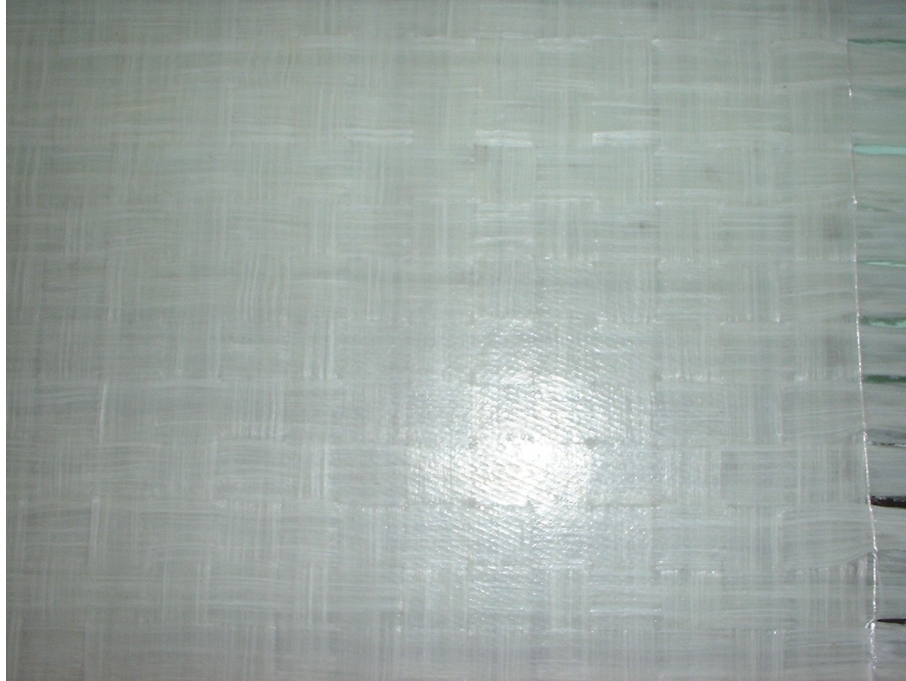
Figure 4-4 Close-up of Consolidated Woven Polypropylene/E-glass
