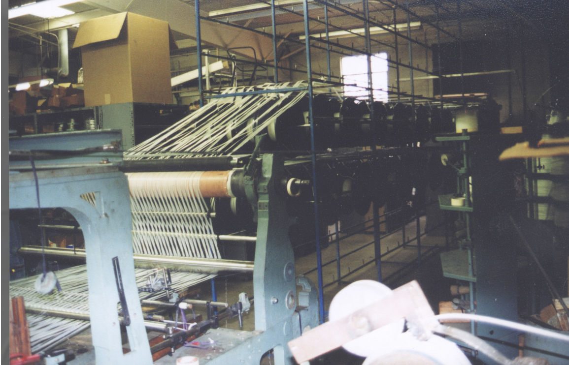
Figure 4.1-1 Picture of Loom Weaving Thermoplastic Prepreg
