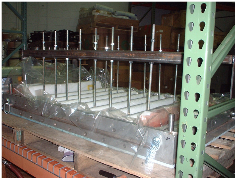
Figure 4.3.2-2 Mold Prepared for Vacuum Bag Thermoforming
