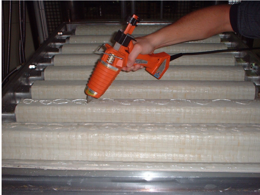
Figure 4.3.2-3 Part Bonding with Low Temperature Melt Adhesive
