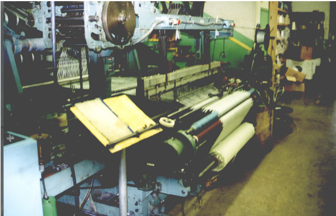
Figure 4.1-2 Take-up Accumulator for Woven Prepreg Fabric
