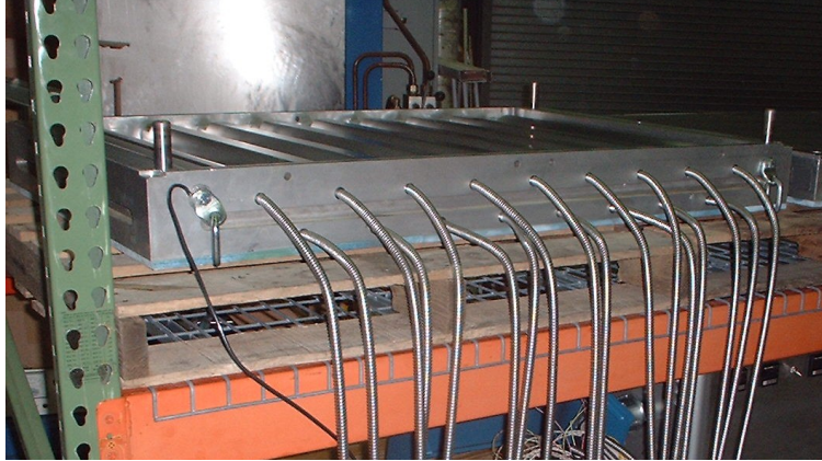
Figure 4.3.2-1 Aluminum Mold Half Showing Inserted Cartridge Heaters
