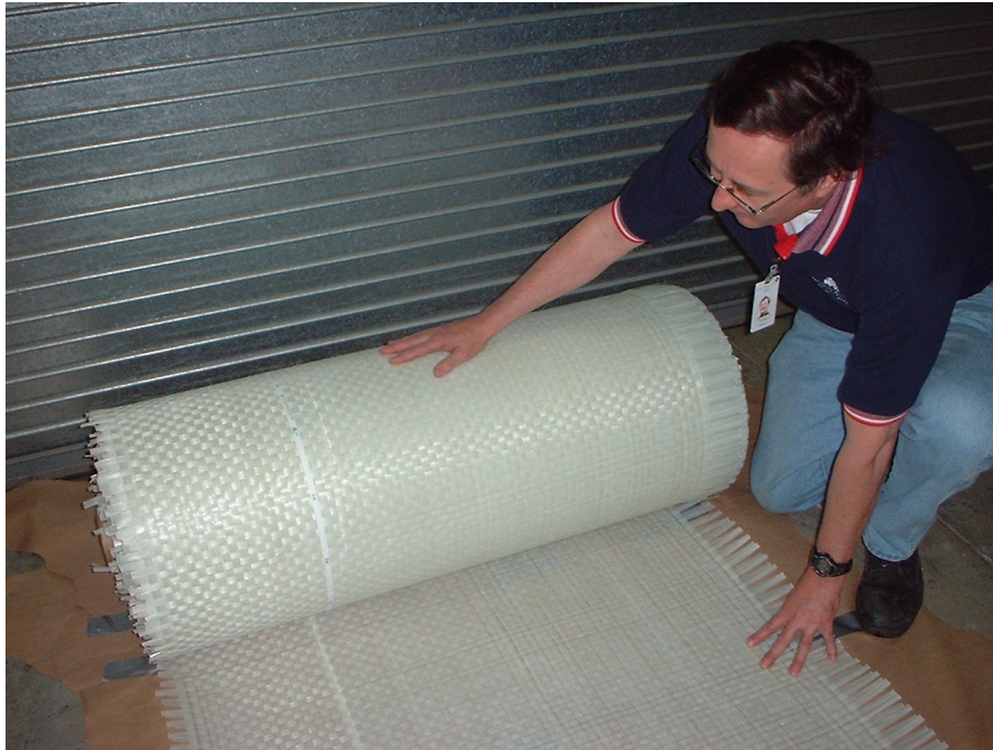
Figure 4-1 Roll of Woven Polypropylene/E-glass Fabric
