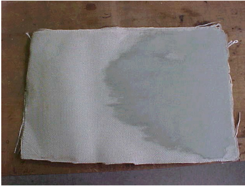
Figure 3.2.1-5 Wet Out Characteristics of Nylon to E-Glass Fiber
