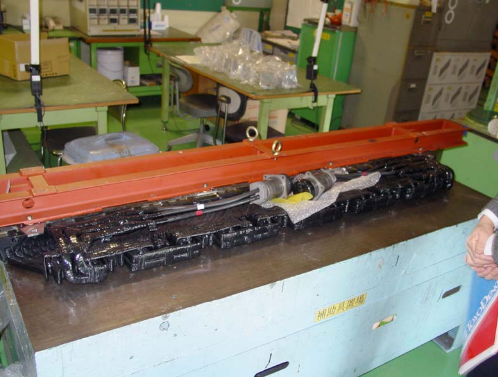
Figure 16. The 100 Series LIM After Painting and Attaching Connectors
