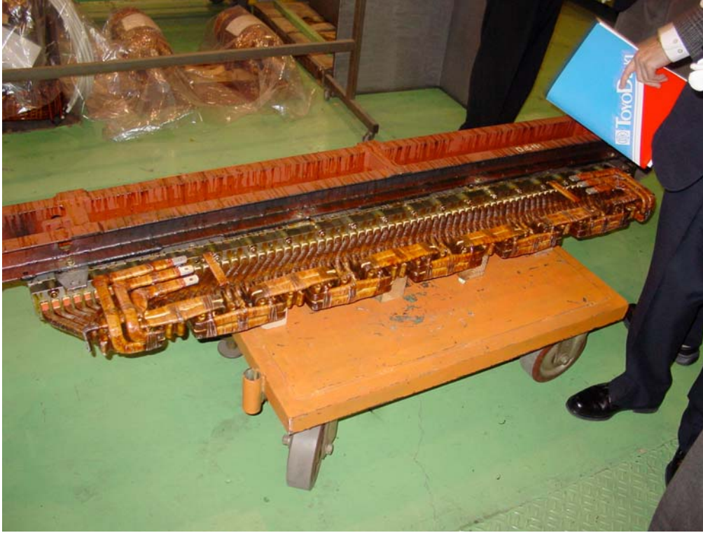
Figure 15. The 100 Series LIM After the Varnishing Process
