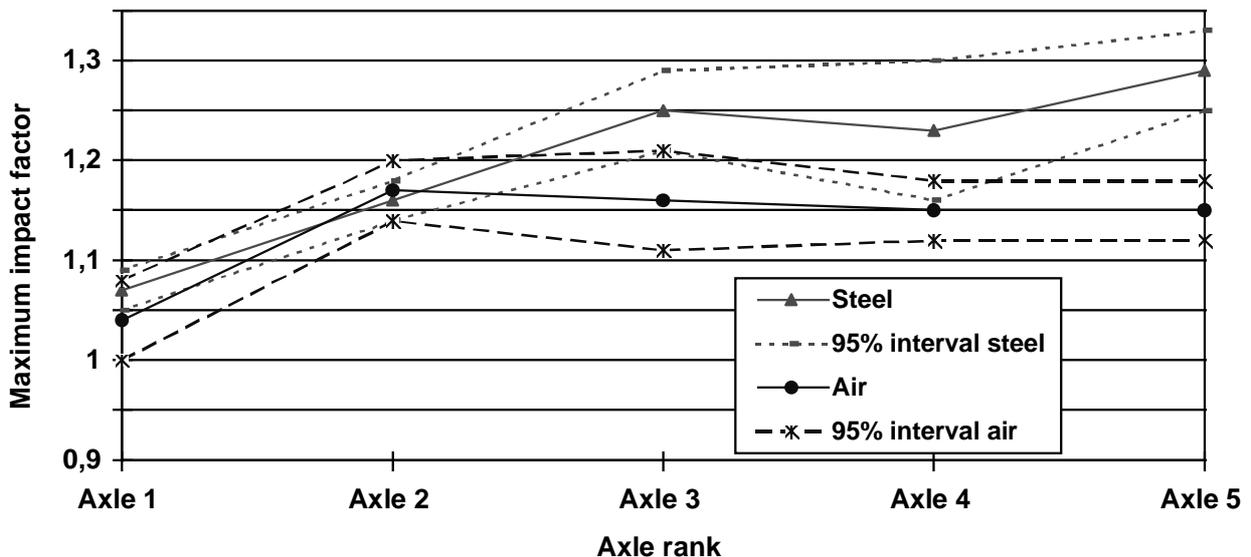
Note: Axles 1 and 2 are either those of 2 axle rigid trucks or belong to the tractor of articulated trucks; axles 3 to 5 are those of the tandem or tridem of the semi-trailers.
