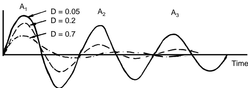
The axle drop tests resulted in the excitation of the unsprung mass, but at times the first cycle contained substantial dynamics from the unsprung mass. In some cases the first peak was not distinguishable and therefore could not be analysed with any degree of confidence. To maximise the potential for comparative analysis, the damping was also calculated using the second and third peaks as well as the third and fourth peaks from the force response curve.
