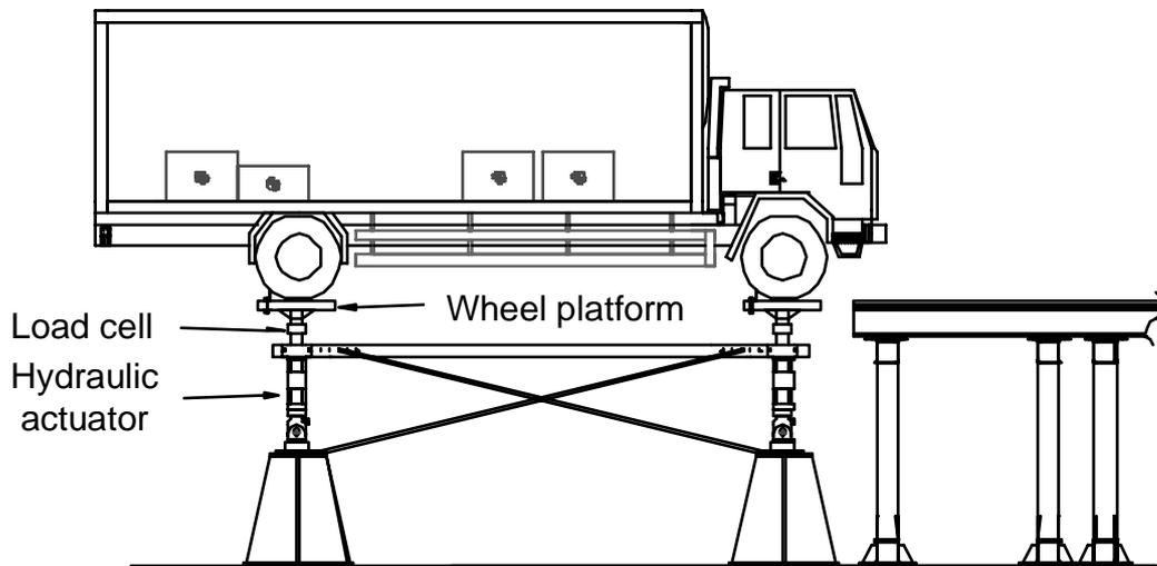
Figure IV.26. NRC instrumented vehicle on NRC shaker
