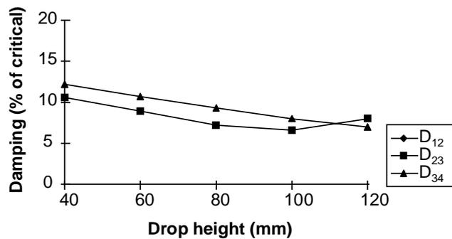
**Figure IV.30. Damping ratio of an air suspension (without dampers): simultaneous axle drop**
