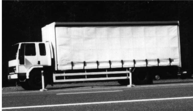
The axle-mounted instrumentation consisted of two strain gauges mounted on the upper and lower surfaces of the axle between the spring and the hub to measure bending strains and two accelerometers to estimate the inertial forces of the axle mass outboard of the strain gauges. The outputs of these transducers could be combined to measure the instantaneous vertical force applied to the road by the wheel on the instrumented axle.
