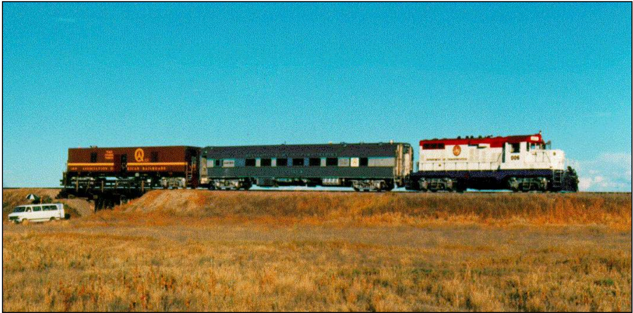
FIGURE 5. Test Train Composed of Locomotive, Instrumentation Car and Track Loading Vehicle at Bridge 101.
