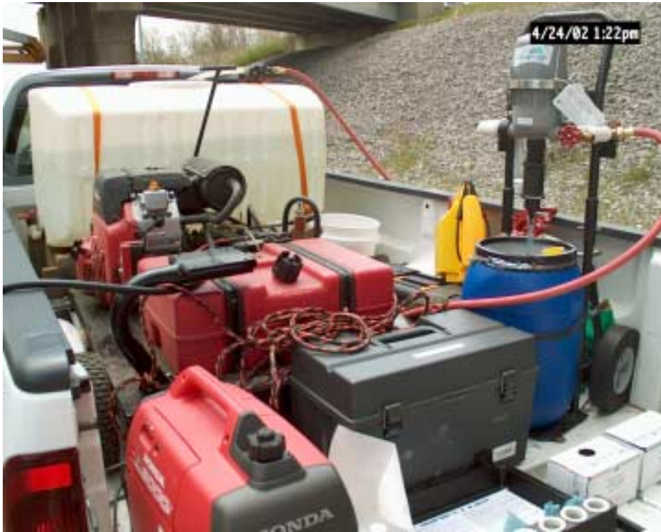
Figure 5 Equipment from CHLOR-RID that pumps the solution for removing invisible salts during pressure washing operation.
