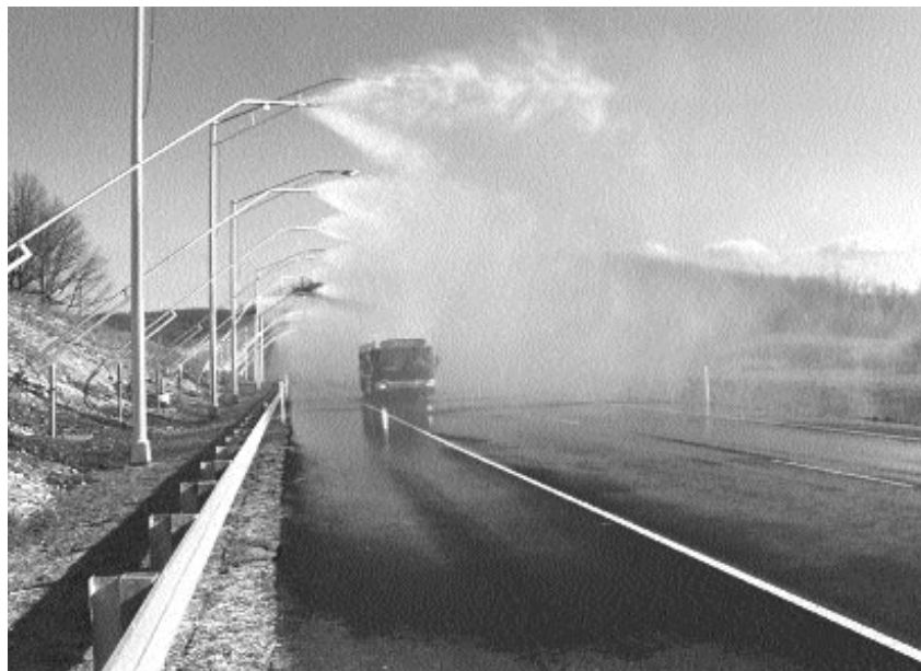
Artificial rain and snow makers provide realistic conditions for tests on the "Smart Road" near Blacksburg.
