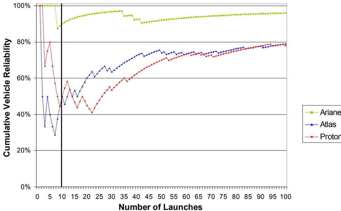
Figure 1: Cumulative Vehicle Reliability for the First 100 Launches
