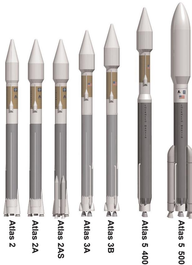
**Figure 3: Atlas Vehicle Lineage**
