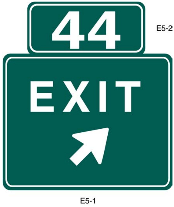
Figure 2E-19. Exit Gore Signs
