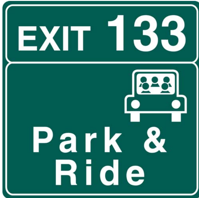
Figure 2E-17. Supplemental Guide Sign for a Park and Ride Facility (Route with Exit Numbering)
