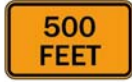
W20-7a 1200 x 1200 mm (48 x 48 in) SUPPLEMENTAL PLAQUE U E 600 x 450 mm (24 x 18 in)
