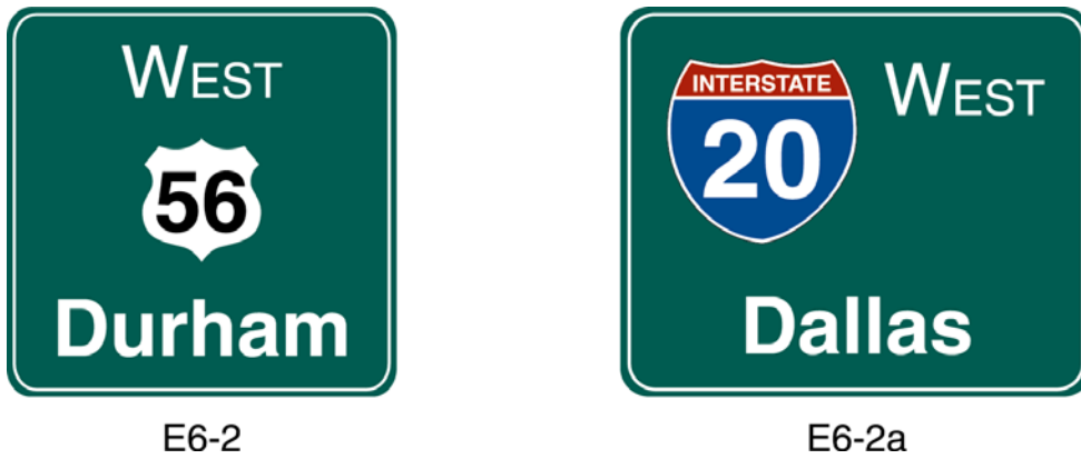
Figure 2E-2. Pull-Through Signs
