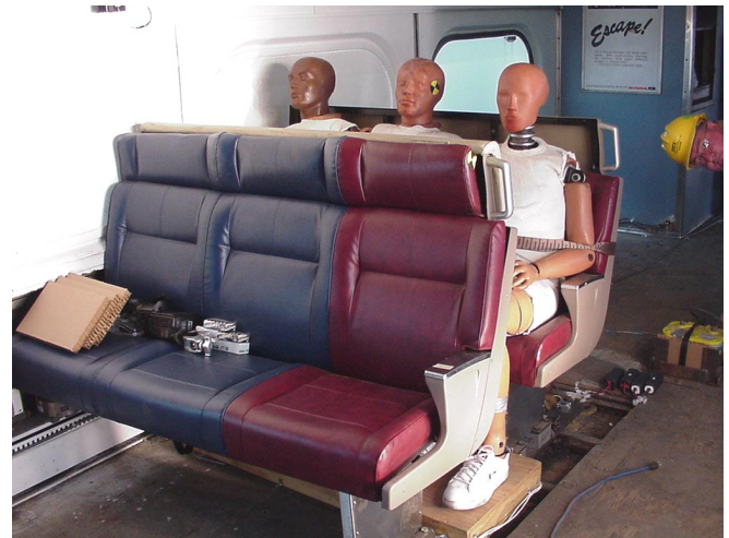
Figure 13. Experiment 1-1, Forward Facing Rows of Seats, Leading Car, Pre-Test
