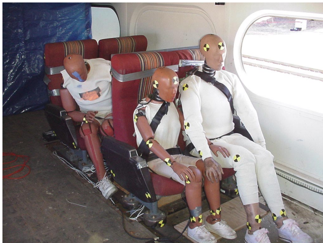
Figure 18. Experiment 1-2, Forward Facing Rows of Seats with Lap and Shoulder Belts, Leading Car, Post-Test
