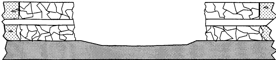
C.) End Section Removal
