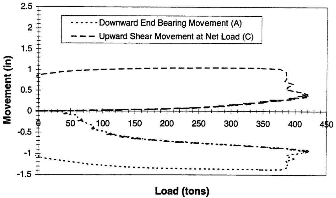
**Figure 4.7a Osterberg Cell Load Movement Curve - Drilled Shaft #3**
