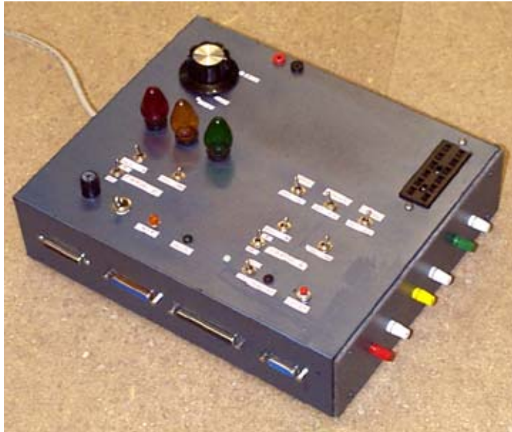
Figure A1-2. Layout of the LED-lamp tester.
