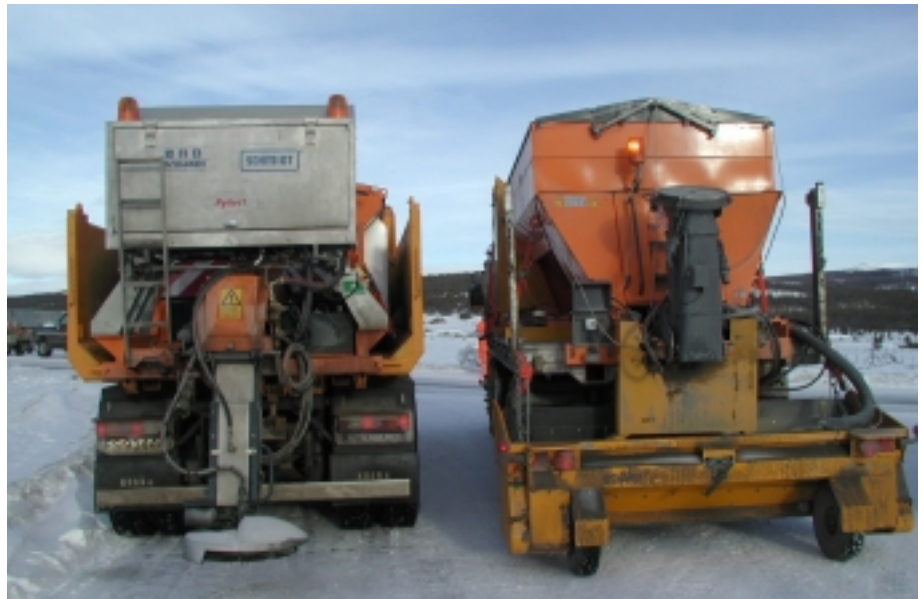
Figure 4. New concept for warm wetted sand. The truck to the left can also be used for spreading salt.
