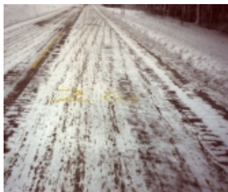
Figure 8. Test field strewn with warm wetted sand on 18 th January 2001. Picture taken on 22 nd January.
