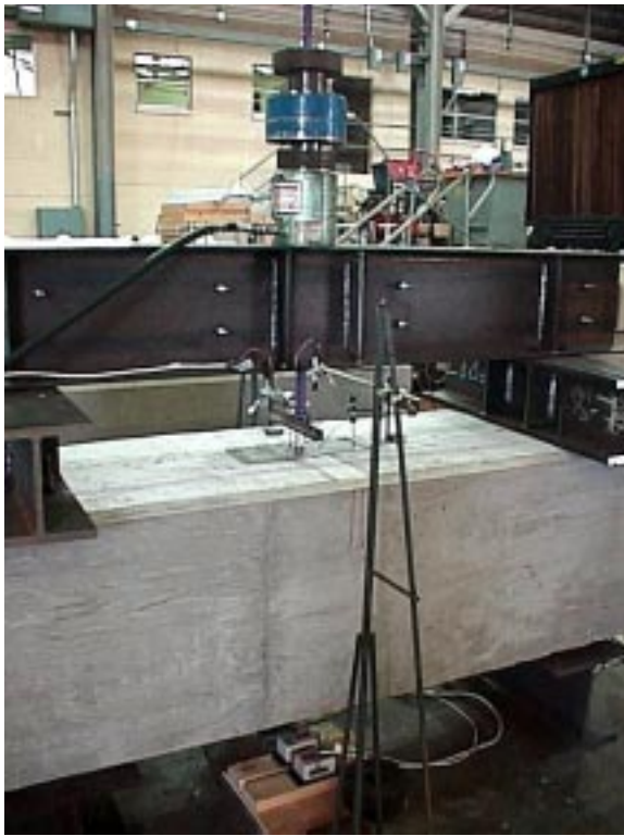
Figure 2 - Setup for Phase 1 Pullout Test
