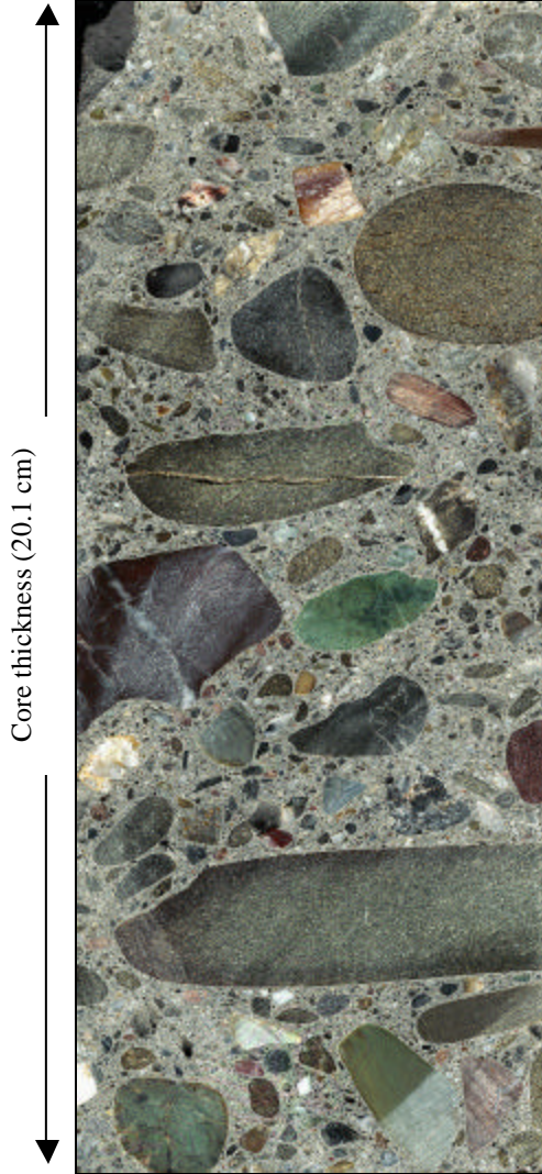
Figure 3.2.4 Polished cross-section of pavement section 06-CS1.
