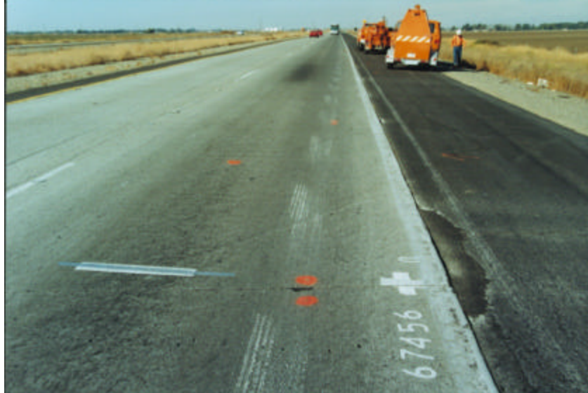
Figure 4.3.1 Overview of the experimental test road at Tracy. Thickened test section 06-7456 with low distress levels.
