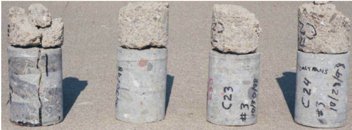
Figure 7.1.2 Eroded CTB at joint. Decreasing erosion moving away from joint (left to right). Experimental test road at Tracy, California, with higher cement content.
