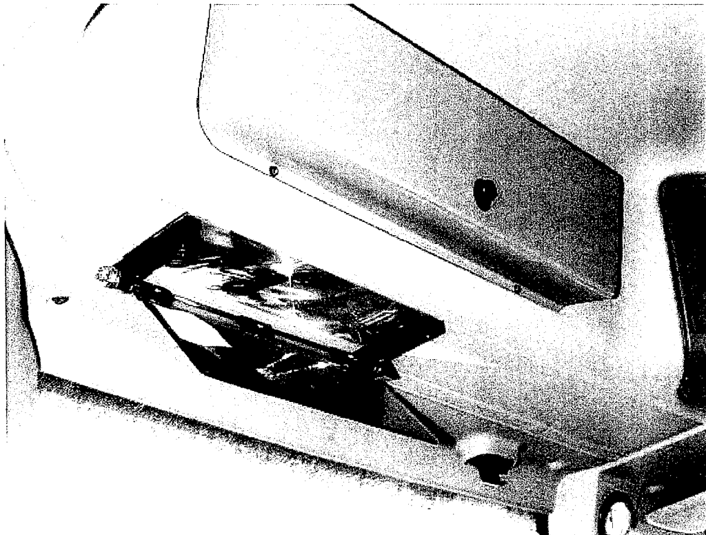
Figure 6. Truck HUD Mounted in Overhead Compartment
