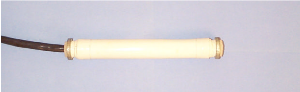
Figure 10.5 Carlson Strain Meter
