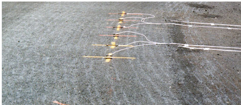
Figure 12.5 Painted Sensor Locations
