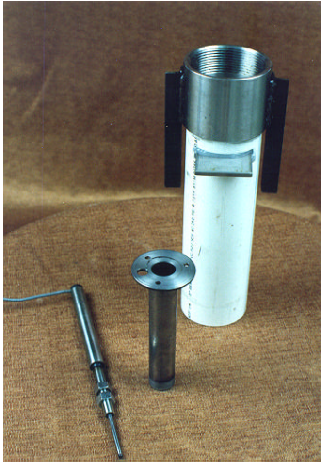
Figure 12.2 Single Layer Deflectometer
