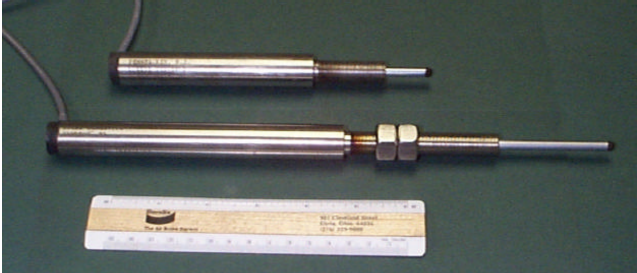
Figure 10.8 Lucas Schaevitz GPD LVDTs
