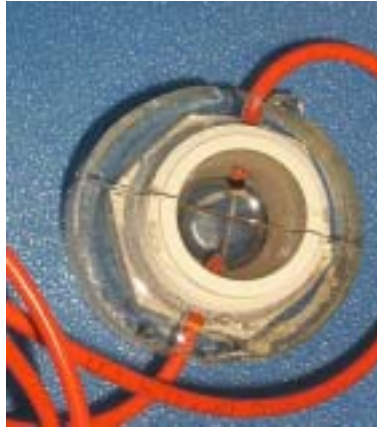
Figure 6. Note that the cap and fiber have been cut. This was achieved using a diamond saw. Into this notch is placed the active chloride sensing element. The fibers act as transmit and receive light pipes.
