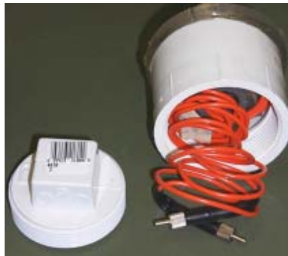
Figure 7. The transmit/receive fibers coil into the base of the sensor unit.
