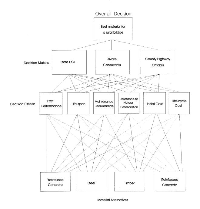
Figure 1. Analytic Hierarchy Model for the Choice of a Bridge Material
