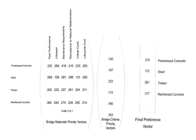
Figure 2. AHP Computation of the Choice of a Bridge Material
