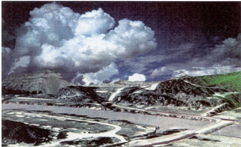
Figure 23. Aerial Photograph Draped Over Digital Elevation Data. Exposed Wire Frame Model Can be Seen at Right Center of Image.
