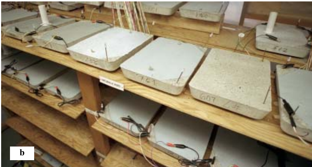
Figure 2.6: Multiple concrete slabs undergoing accelerated electrochemical aging in a controlled humidity enclosure: (a) overall view; (b) close-up of concrete slabs
