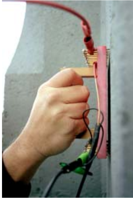
Figure 3.12: Oregon DOT resistance probe for measurement of anode coating resistivity
