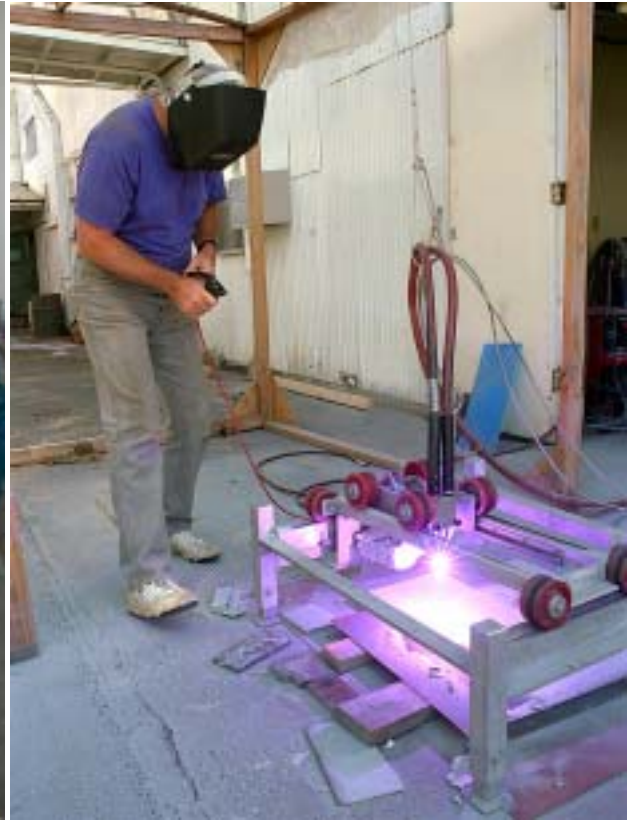
Figure 2.4: Oregon DOT robotic x-y traversing system used to apply TS Zn anode to concrete slabs
