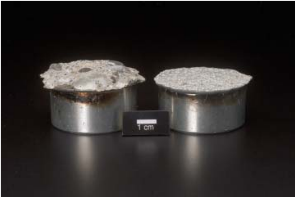
Figure 4.13: Pullout of concrete as a result of bond strength tests for bare concrete (left) and TS Zn coated concrete (right)
