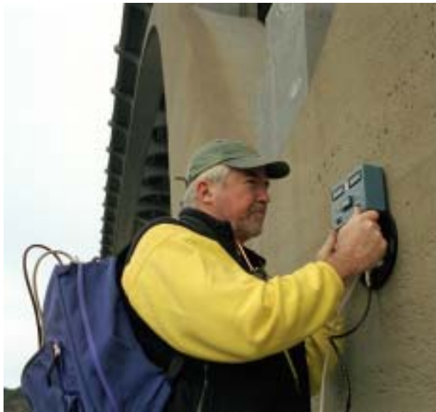
Figure 3.13: Portable surface air permeability instrument in use
