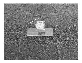
Figure 5: LDP gauge and installation details
