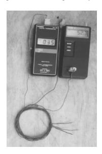
Figure 4: Temperature probes and thermocouple wires
