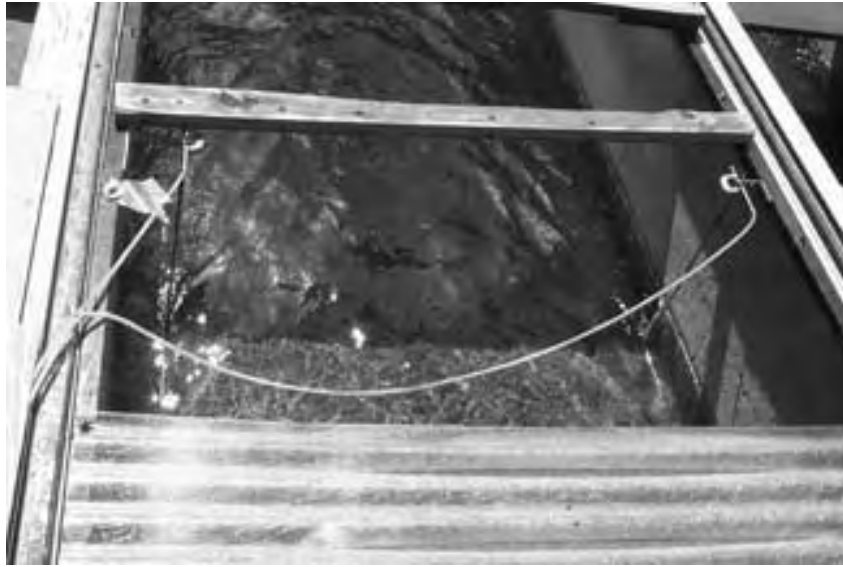
Figure 4.5: Two Pitot tubes in the channel while the water is flowing
