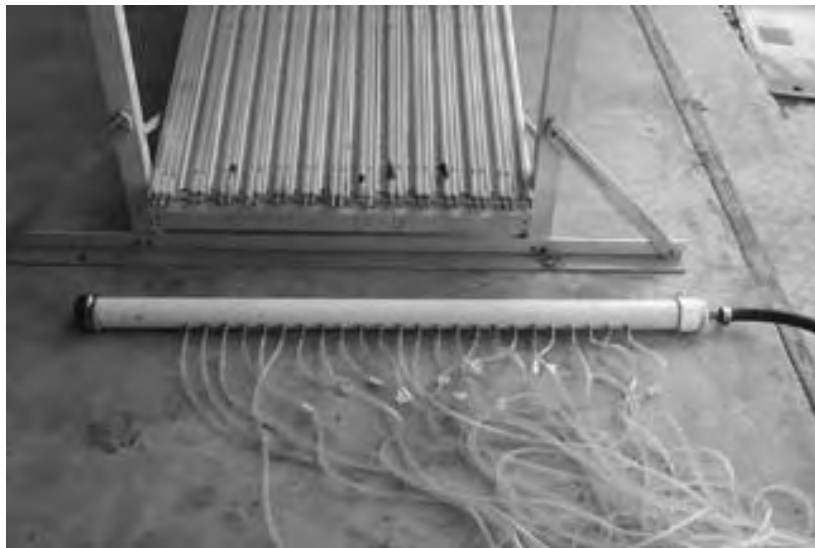
Figure 4.4: The flushing process of the 24 tubes
