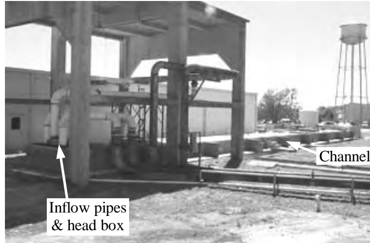
Figure 3.1: Overview of the physical model showing the channel and the pipes that supply the flow
