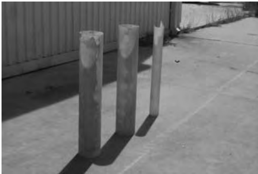
Figure 3.6: Photograph showing the roughened piers: two 6.5 in. (16.5 cm) piers and one 3.5 in. (8.9 cm) pier
