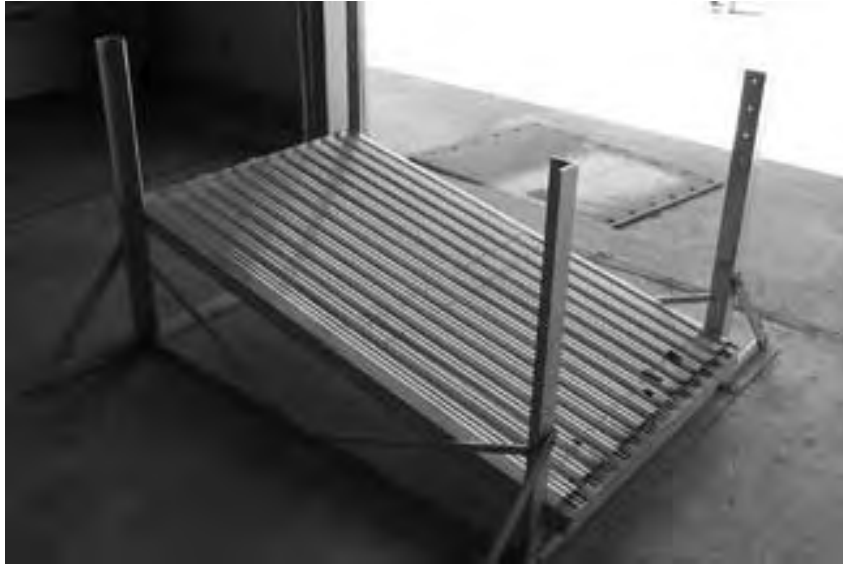
Figure 3.16: Manometer board having twenty-four tubes and a slope of 1/5
