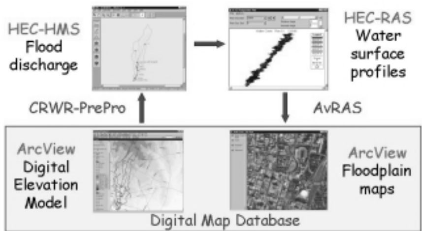
Figure 1: Framework of hydrologic and hydraulic modeling using GIS.
