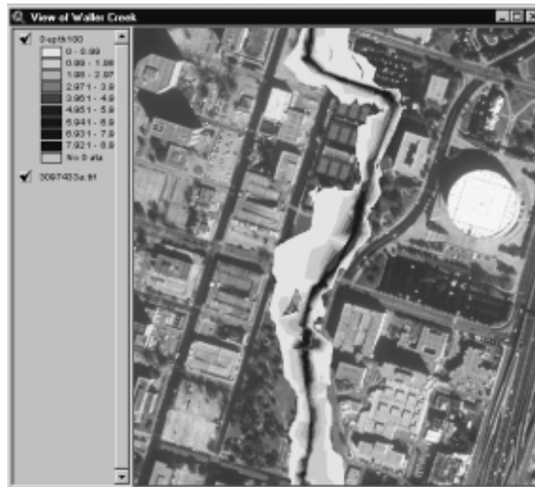
Figure 10: Floodplain (in blue) overlaid on the digital orthophoto of downtown Austin, Texas. Dark blue corresponds to deep areas.
