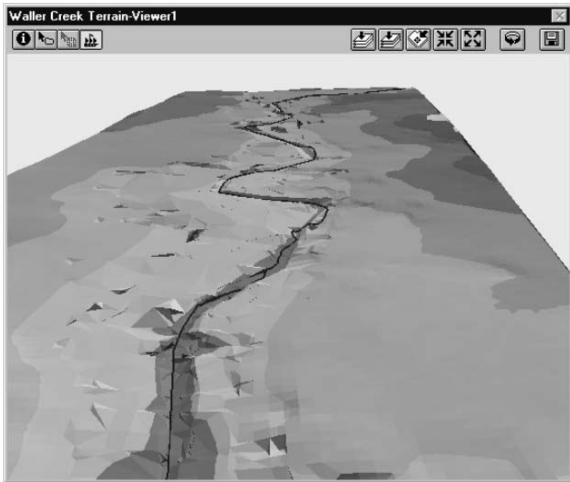
Figure 3.14 Waller Creek Terrain TIN
